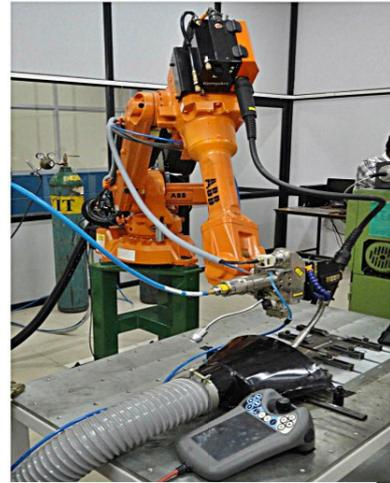
Fig. 1 Laser Welding Setup
