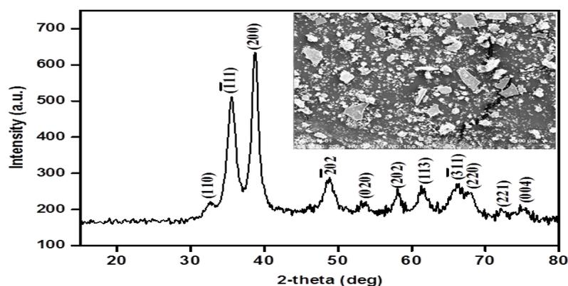
**Figure 1.** XRD patterns and SEM images (Inset) of synthesized copper oxide nanoparticles.
