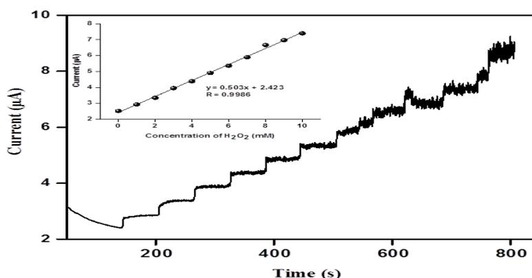
**Figure 4.** Amperometric response for the detection of H<sub>2</sub>O<sub>2</sub>. *Inset* shows the corresponding calibration plot.
