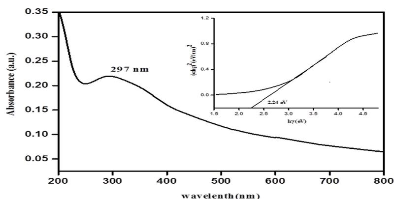
**Figure 2.** UV-vis absorption spectrum of monoclinic CuO. *Inset:* shows the plots of  $(\alpha E_{\text{photon}})^2$  vs.  $E_{\text{photon}}$ .
