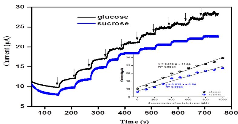
**Figure 3.** Chronoamperometry response of glucose and sucrose with glassy carbon modified with CuO in 0.1 M NaOH solution at a regular interval of 60 s. *Inset (right)* the corresponding calibration plot of net current vs. concentration.
