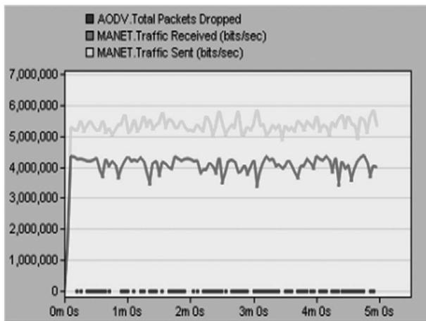
Figure 5. Normal network model: Time (s) vs. Number of packets (bits/sec).
