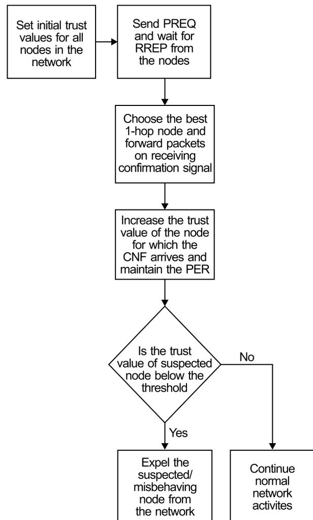
Figure 4. Flowchart of Secure BEFORE routing scheme.
