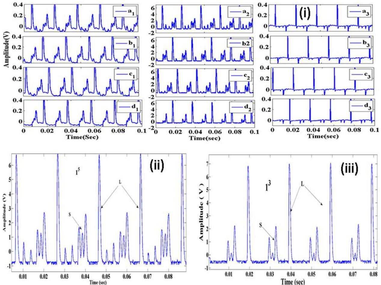
FIG. 2. (i) Signal of the floating potential fluctuations obtained by the inner (a<sub>1</sub>)–(d<sub>1</sub>), the middle (a<sub>2</sub>)–(d<sub>2</sub>), and the outer Langmuir probes (a<sub>3</sub>)–(d<sub>3</sub>) in various magnetic fields: (a) 0 G, (b) 4 G, (c) 8 G, and (d) 12 G at 240 V. (ii) and (iii) Shows the expanded view of the signals a<sub>2</sub> and d<sub>2</sub> of (i).
