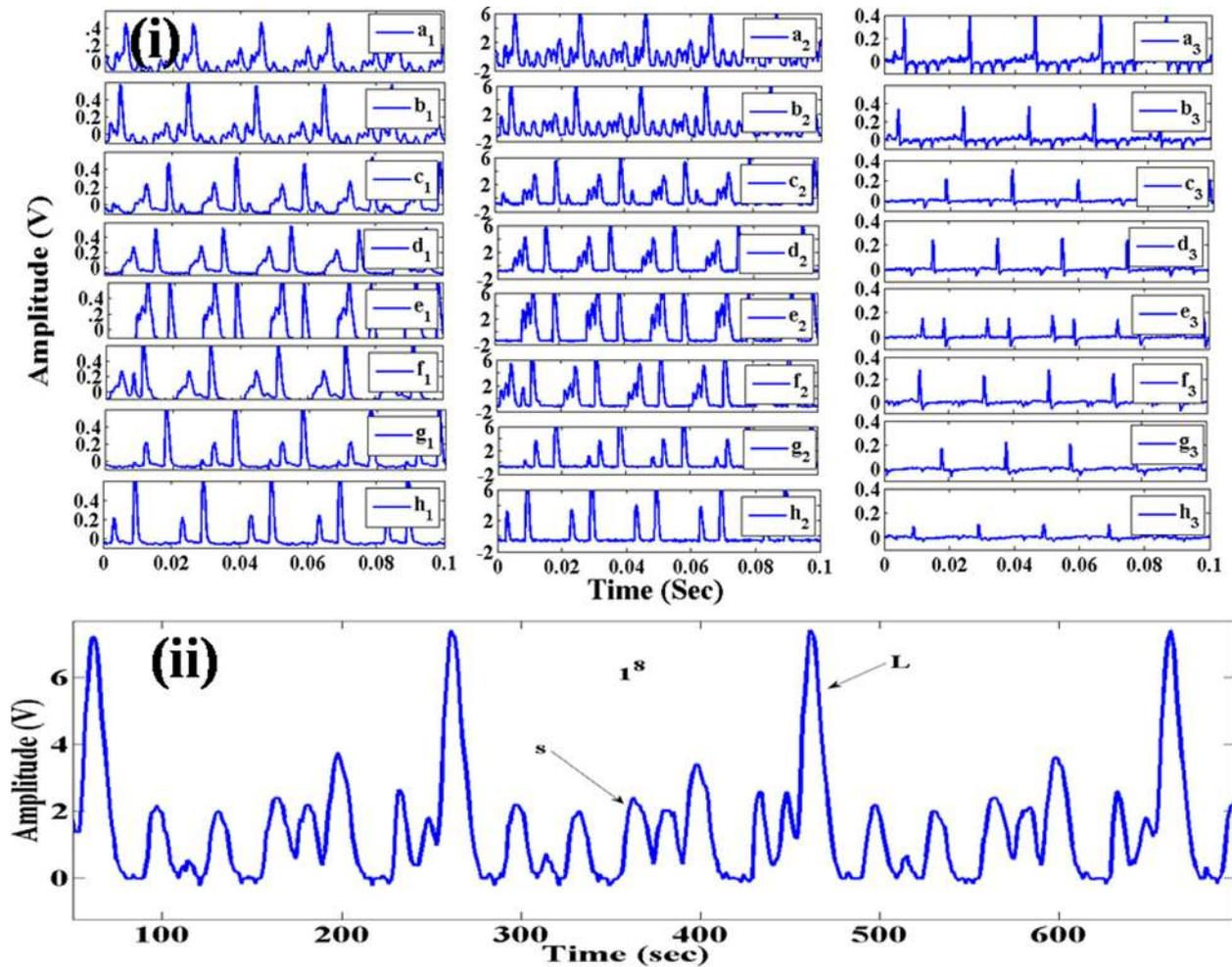
FIG. 3. (i) Represents the time series of the floating potential fluctuations obtained by the inside ( $a_1$ )–( $h_1$ ), the middle ( $a_2$ )–( $h_2$ ), and the outside Langmuir probes ( $a_3$ )–( $h_3$ ) in various magnetic fields: (a) 0 G, (b) 23 G, (c) 70 G, (d) 76 G, (e) 90 G, (f) 132 G, (g) 164 G, and (h) 198 G. (ii) Representation (Zoom) of the signal  $a_2$  at 250 V.
