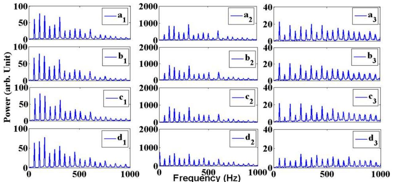
FIG. 5. FFT power spectra of the signals of the floating potential fluctuations in regimes I, II, and III at 240 V.
