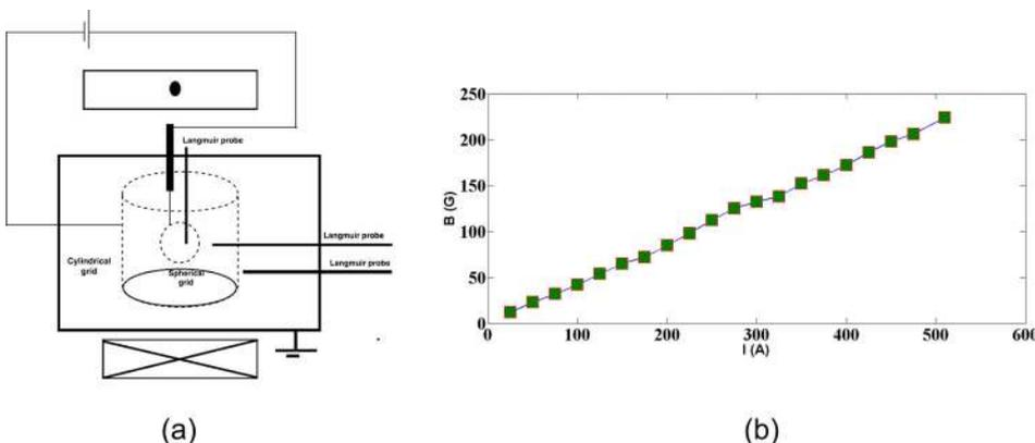
FIG. 1. (a) Schematic diagram of the experimental setup. (b) Calibration curve for the current passes through the Helmholtz coil versus the produced magnetic field.
