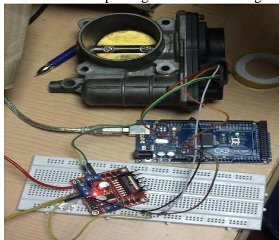
**Figure 2.** Experimental Setup for Electronic Throttle Control
