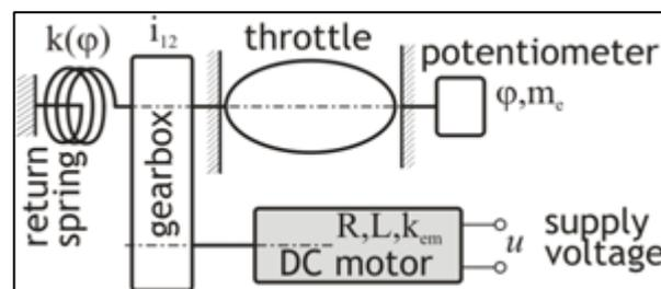
**Figure 1.** Schematic Diagram of an Electronic Throttle Control [17]
