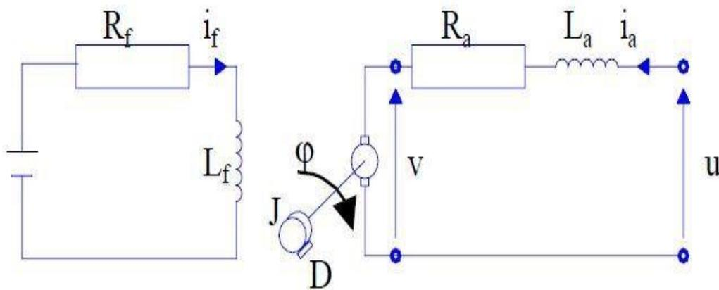
**Figure 3.** Linear Model for Electronic Throttle Control [16]
