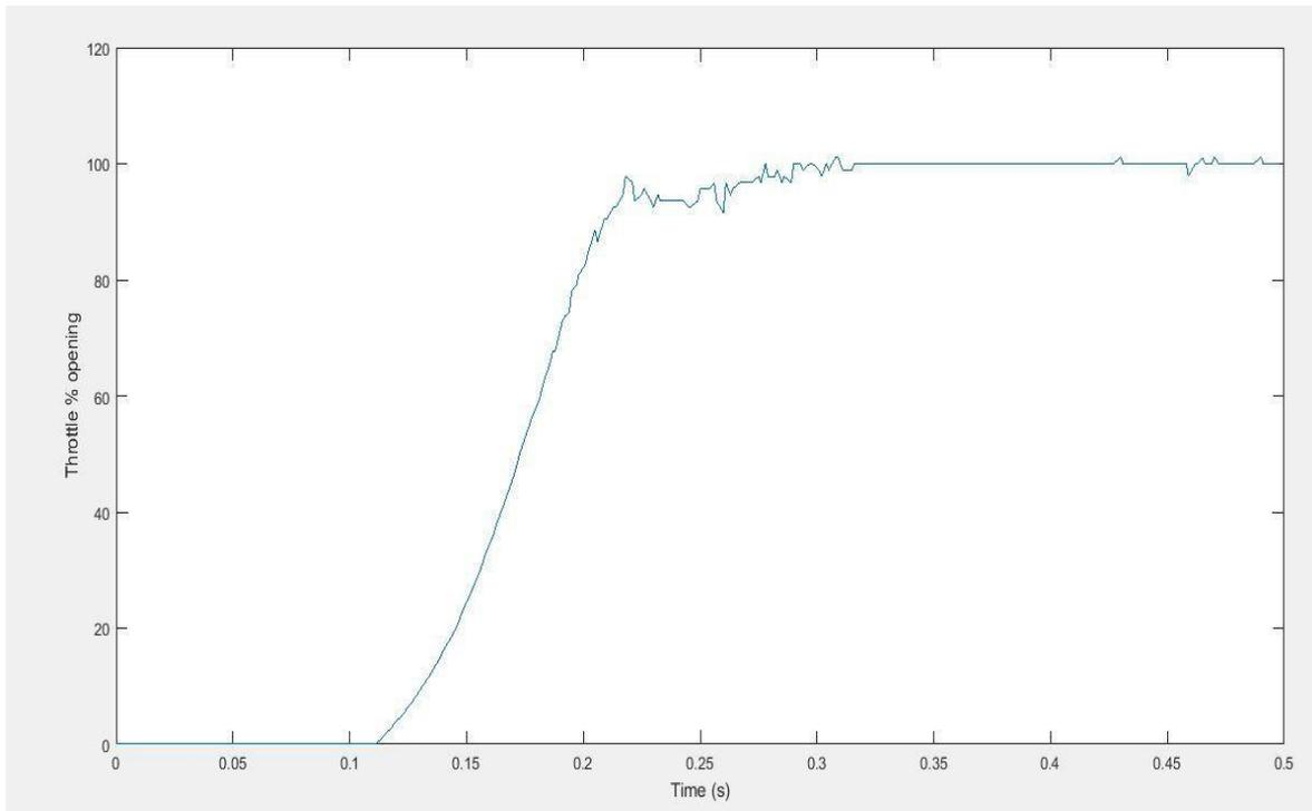
**Figure 6.** Percentage of Throttle Opening v/s Time plotted in MATLAB for ETB (Linear Condition)
