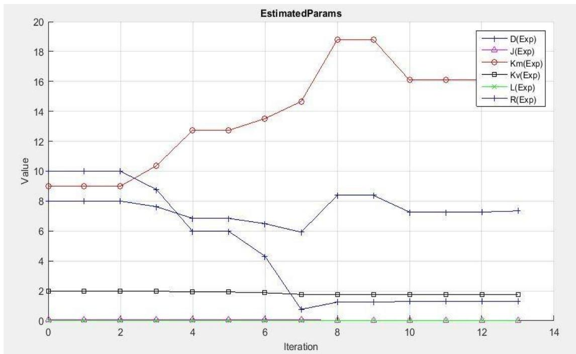
**Figure 12.** Convergence plot of the estimated parameters
