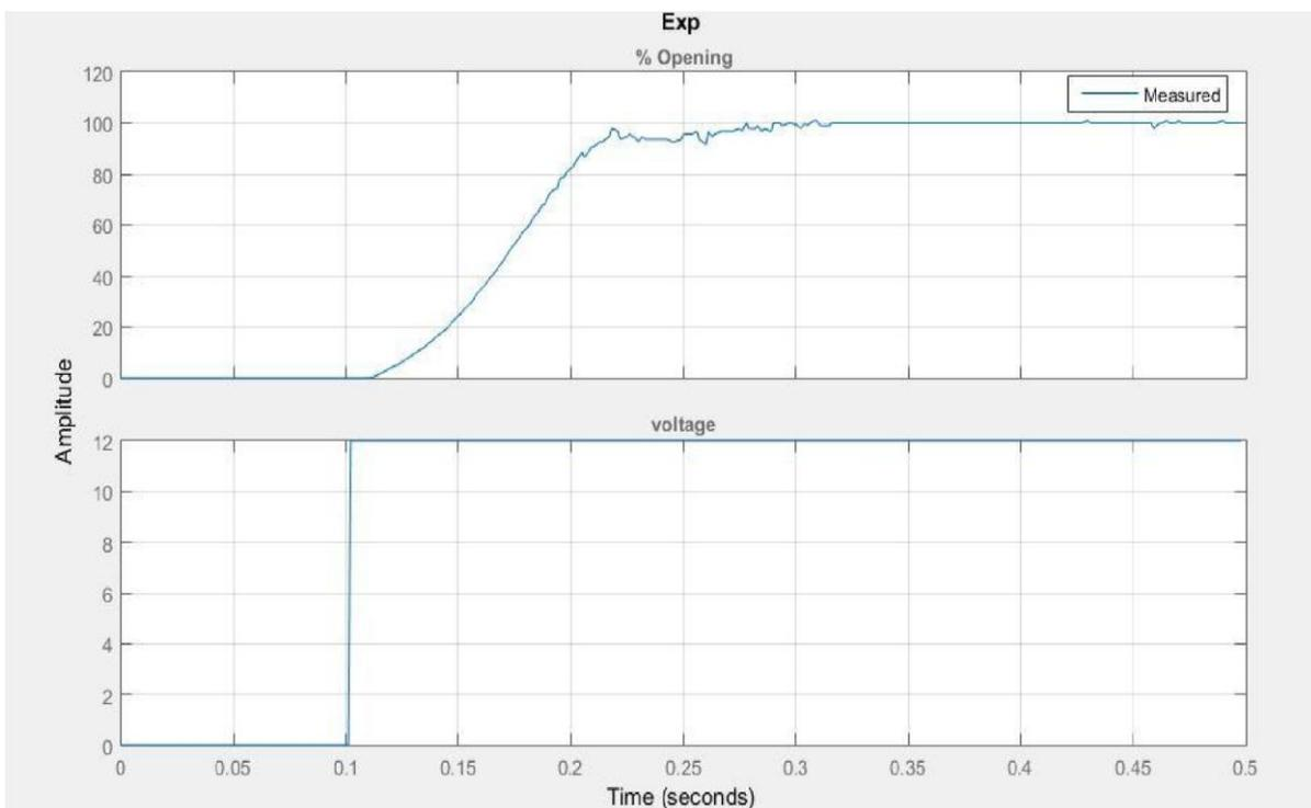
**Figure 7.** Percentage of Throttle Opening and Step input v/s Time plotted in MATLAB for ETB (Linear Condition)
