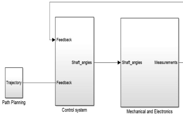
Figure 7: Simulink model of the Robot System.
