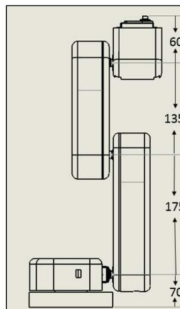
Figure 1: Robotic Arm Structure (dimensions in mm)
