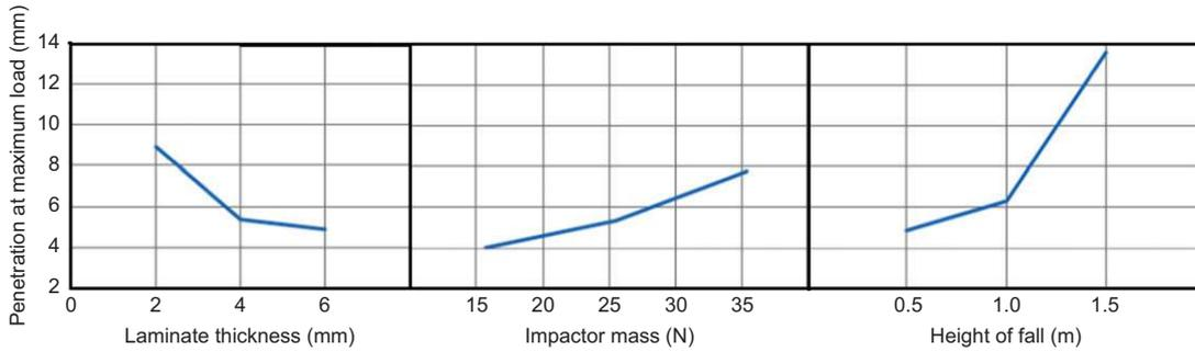
Figure 8 Illustration of factor effects on penetration.
