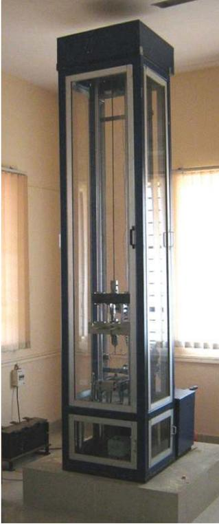
Figure 1 Instrumented falling-weight impact test equipment.
