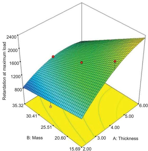
**Figure 7** Effect of impactor mass and thickness on retardation.
