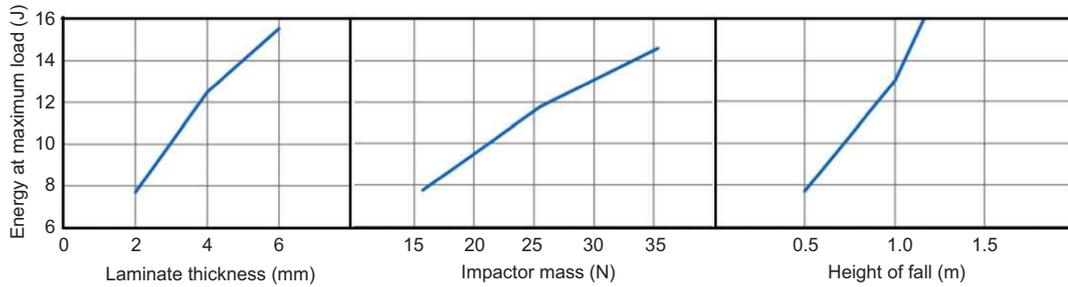
Figure 10 Illustration of factor effects on absorbed energy.
