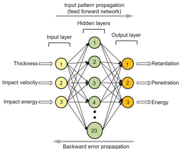
Figure 3 Architecture of a multilayer perceptron: feed-forward network with backward propagation error (3-20-3).
