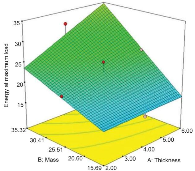
Figure 11 Effect of impactor mass and thickness on energy at maximum load.
