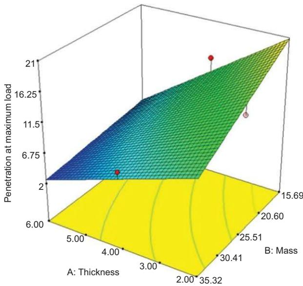
Figure 9 Effect of impactor mass and thickness on penetration.
