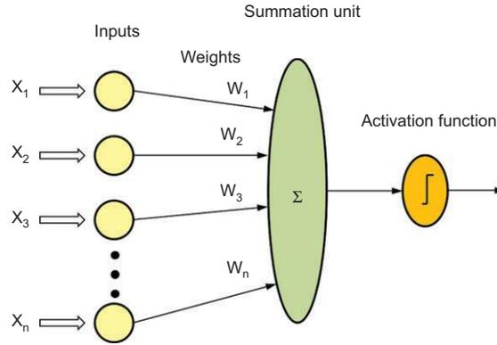
Figure 2 Structure of an artificial neuron.
