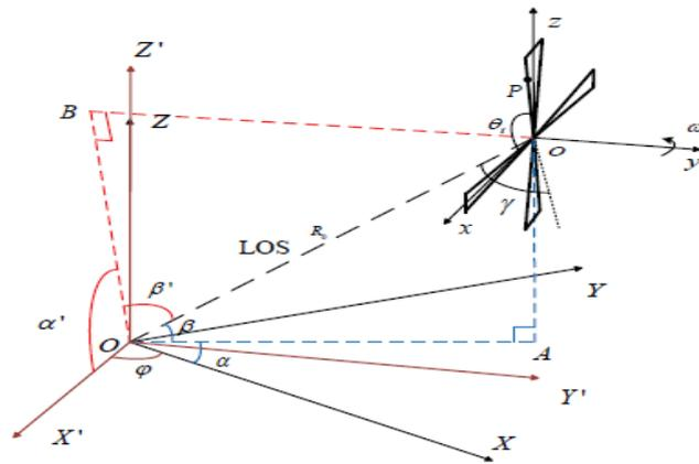
**Figure 1.** Rotor in Radar coordinate system
