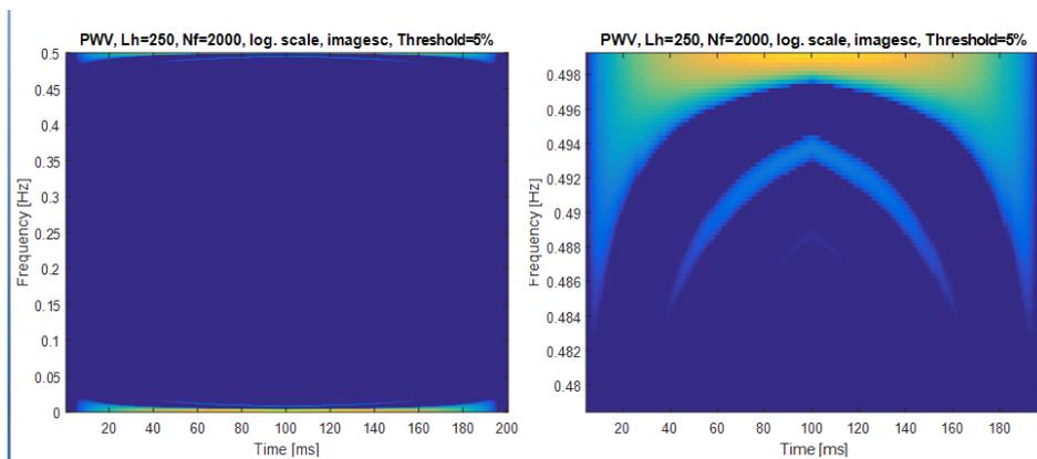
**Figure 5.** pseudo-WVD spectrum of the received signal (image to the right is the magnified version of spectrum's positive peak)
