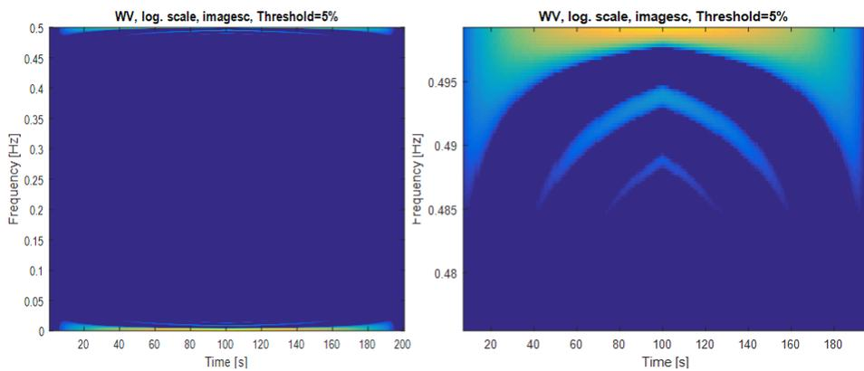
**Figure 4.** WVD spectrum of received signal (image to the right is the magnified version of spectrum's positive peak)
