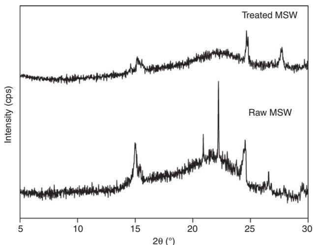
Figure 4 XRD of raw and treated MSW.
