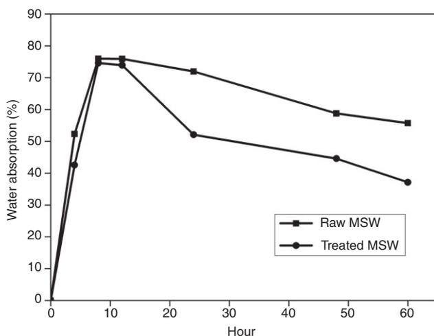
**Figure 8** Water absorption properties of raw and treated MSW.
