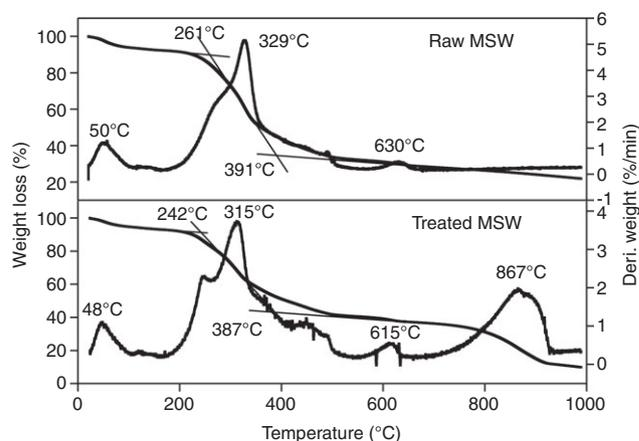
Figure 6 TG/DTG of raw and treated MSW.
