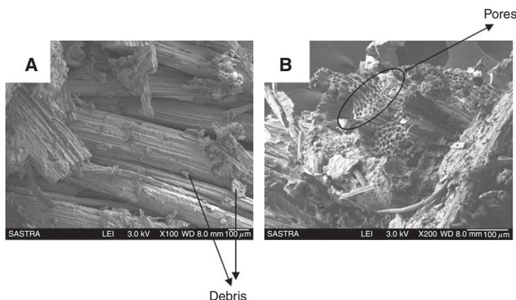
**Figure 9** Scanning electron images of the tensile fracture surface of composites at (A) 20%  $V_f$  of filler loading, (B) 40%  $V_f$  of filler loading (ratio of MSW/banana fiber=50:50).
