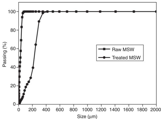
**Figure 3** Particle size distribution of raw and treated MSW.
