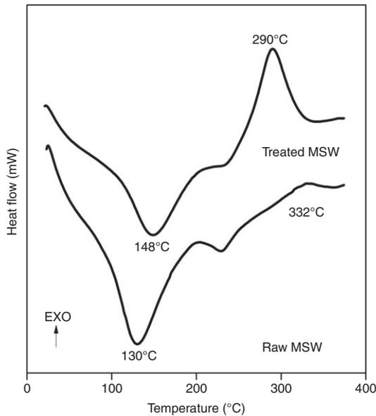
**Figure 7** DSC thermograms of raw and MSW.
