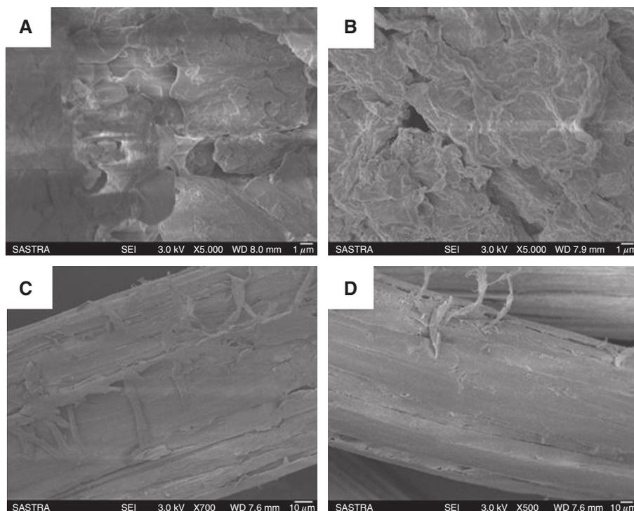
Figure 2 SEM micrograph of (A) raw MSW, (B) treated MSW, (C) raw banana fiber and (D) treated banana fiber.
