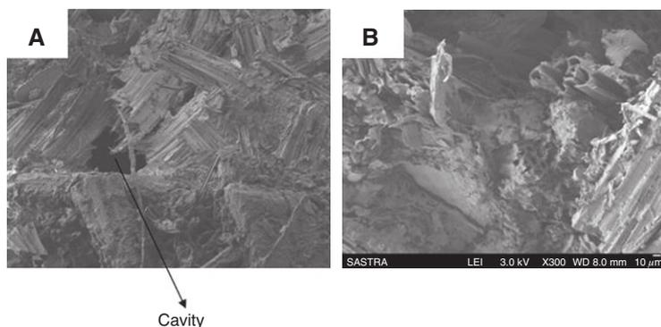
**Figure 10** SEM images of tensile fracture surface of (A) untreated and (B) chemically treated MSW/banana fiber composites (ratio of MSW/banana fiber=50:50).
