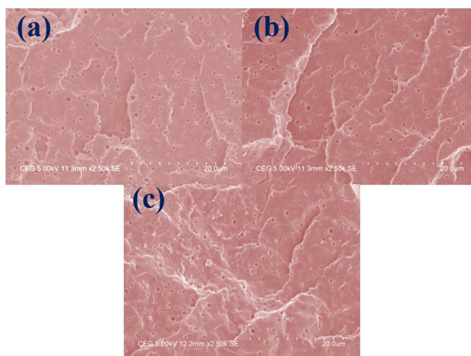
**Fig. 3:** SEM micrographs of cryofractured and etched (a) PASP (b) PASP+1 wt. % HNTs (c) PASP+1 wt. % mHNTs
