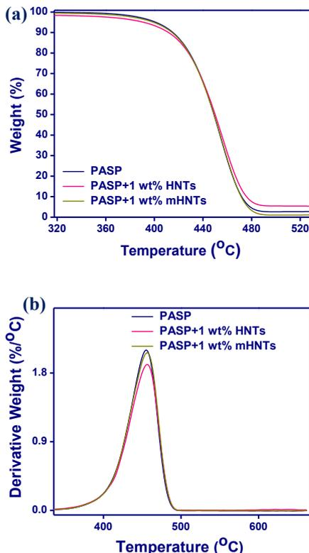
**Fig. 9:** (a) TGA and (b) DTG curves of PASP, PASP+1wt% HNTs, PASP+1wt% mHNTs
