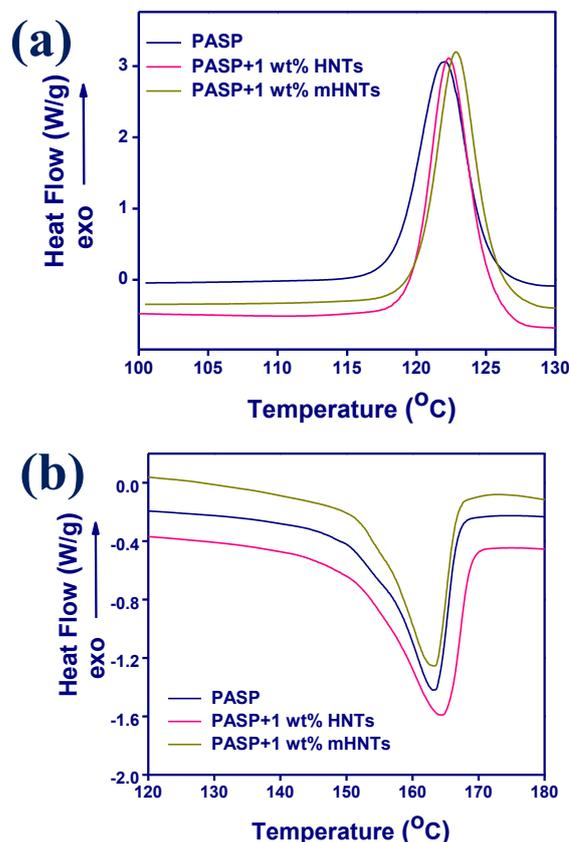
**Fig. 4:** DSC (a) crystallization exotherms and (b) melting endotherms of PASP, PASP+1wt%. HNTs and PASP+1wt%. mHNTs
