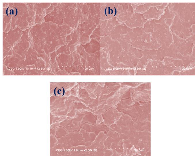
Fig 8: Impact fractured SEM micrographs of (a) PASP (b) PASP+1 wt% HNTs (c) PASP+1 wt% mHNTs
