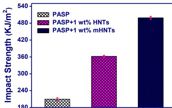
Fig. 7: Impact strength of PASP, PASP+1wt%. HNTs, PASP+1wt%. mHNTs
