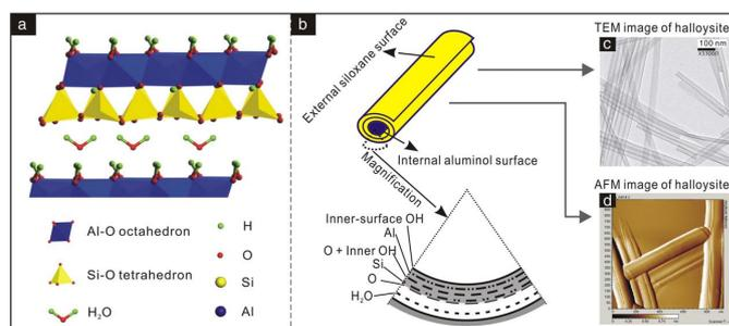
**Fig. 1:** Schematic diagram of (a) crystalline structure of HNTs- (10 Å), (b) structure of HNTs particle, (c, d) TEM and AFM images of HNTs [23].
