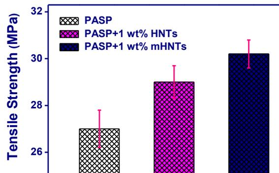
Fig. 6: Tensile strength of PASP, PASP+1wt%. HNTs, PASP+1wt%. mHNTs
