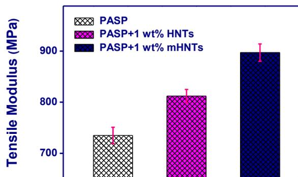
Fig. 5: Tensile modulus of PASP, PASP+1wt%. HNTs, PASP+1wt%. mHNTs
