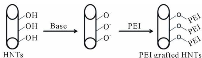
**Fig. 2:** Schematic representation of the surface treatment of HNTs [34].
