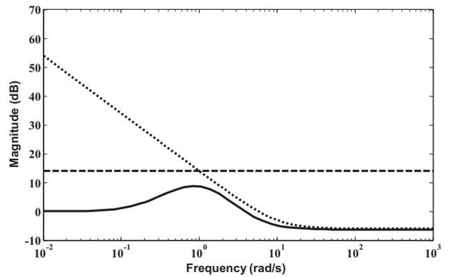
Fig. 14. Magnitude plot of complementary sensitivity function  $T_d(j\omega)$  (solid),  $1/l_m(j\omega)$  for  $\Delta\theta_p = 0.25$  (dot),  $1/l_m(j\omega)$  for  $\Delta k = 0.2$  (dash).
