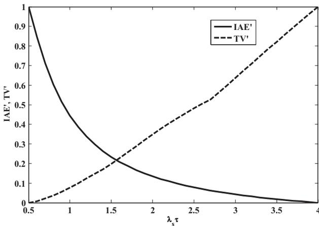
Fig. 5. Variation of IAE and TV for servo loop with respect to  $\lambda_s$ .
