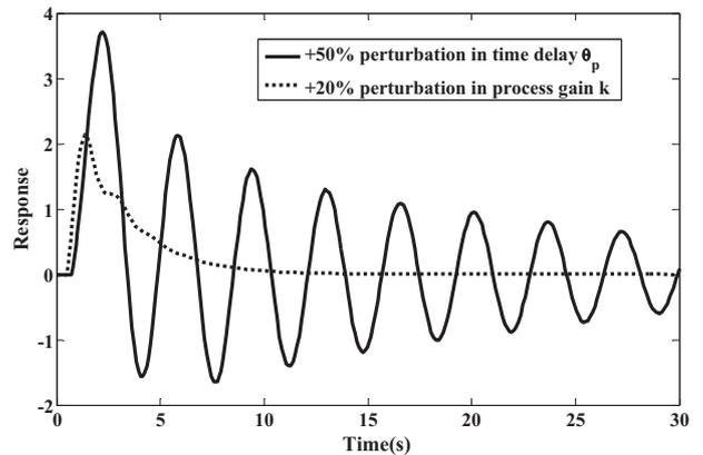
Fig. 16. Robust performance analysis of Example 2 for perturbations in process gain and time delay.
