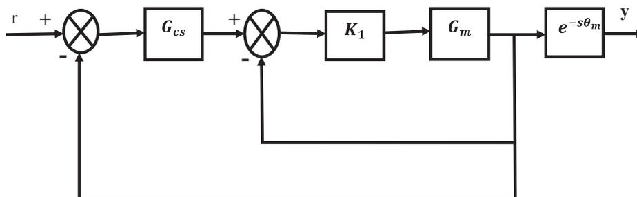
Fig. 2. Block diagram representation of servo response.
