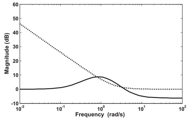
Fig. 15. Magnitude plot of complementary sensitivity function  $T_d(j\omega)$  (solid),  $1/l_m(j\omega)$  for  $\Delta\tau = -0.5$  (dot).
