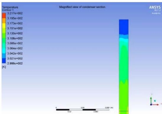
Figure 2a. Temp. profile of ammonia heat pipe.
