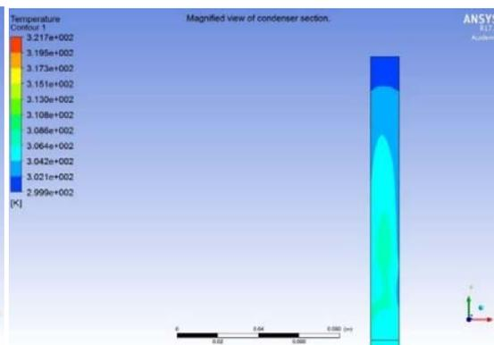
Figure 2b. Temp. profile of water heat pipe.
