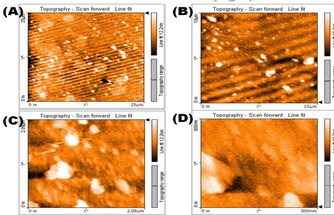
**Figure 8: AFM images of CuNPs (A) 25 μm (B) 10 μm (C) 2.09 μm (D) 800nm**
