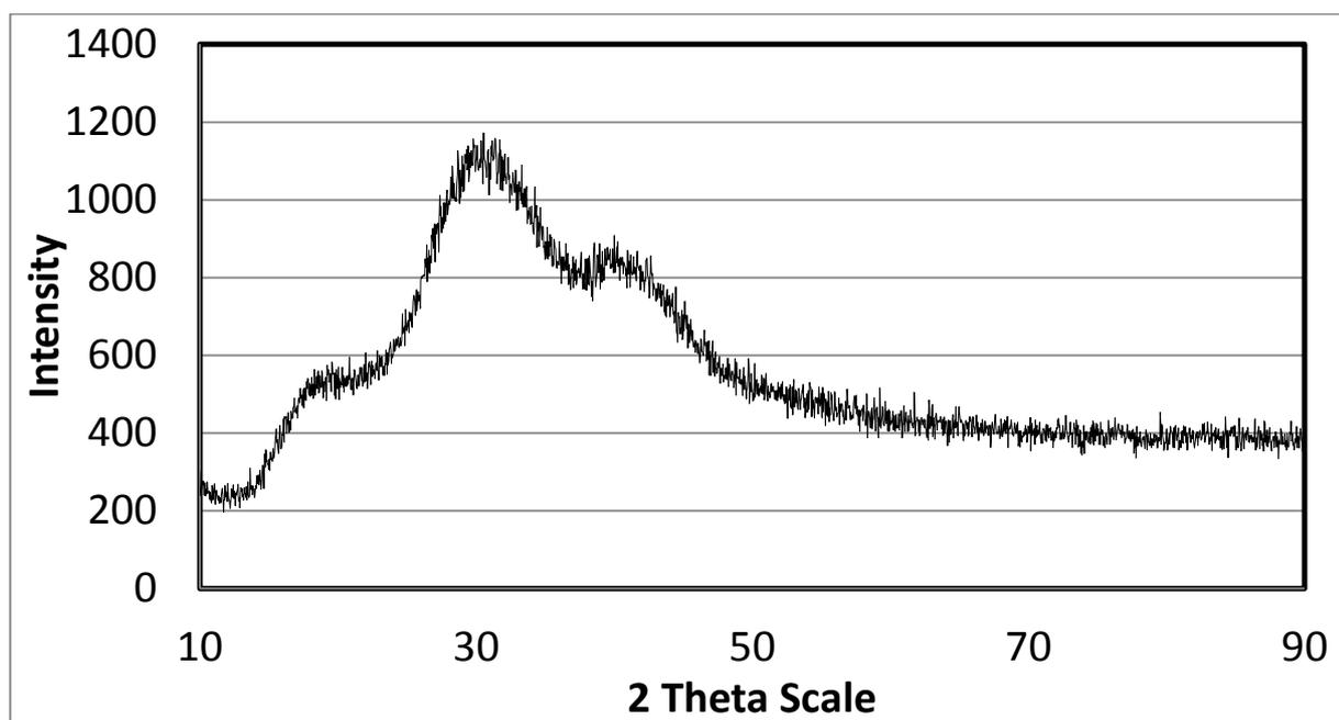
Figure 5 : XRD spectrum of Cu NP
