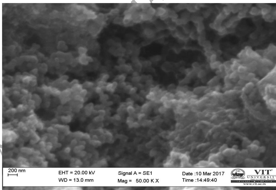
Figure 6: SEM images of copper nanoparticles synthesized using *Persea americana* seed extract
