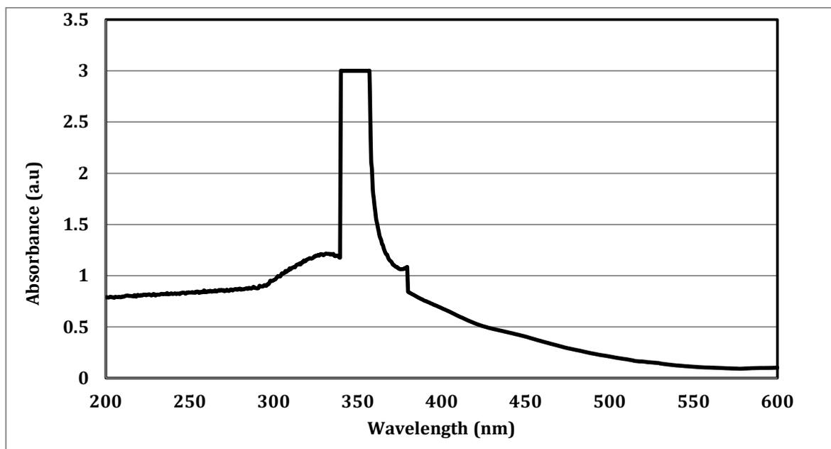
Figure 2. UV- Vis spectra of Cu nanoparticles
