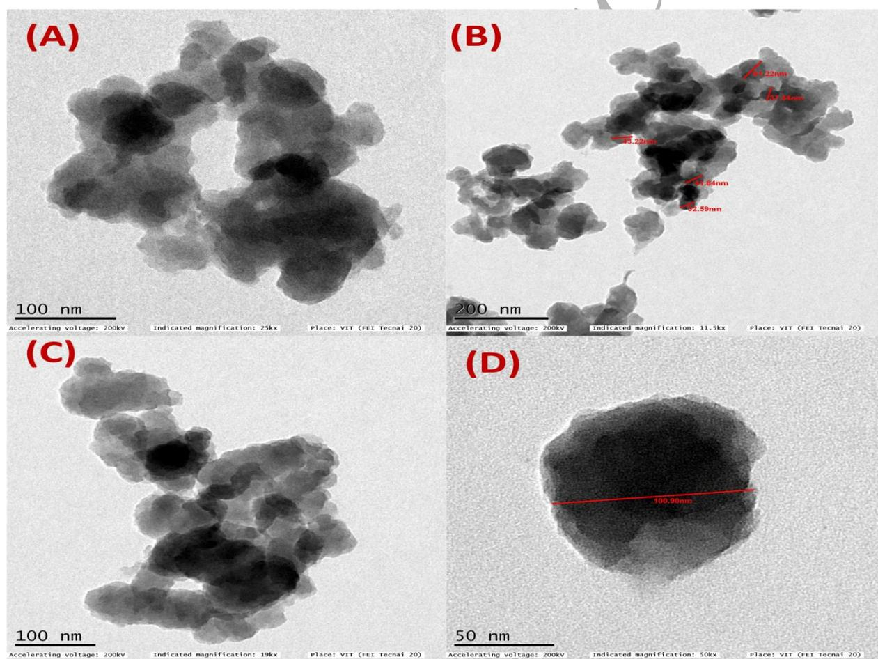
Figure 7: TEM Images of copper nanoparticles
