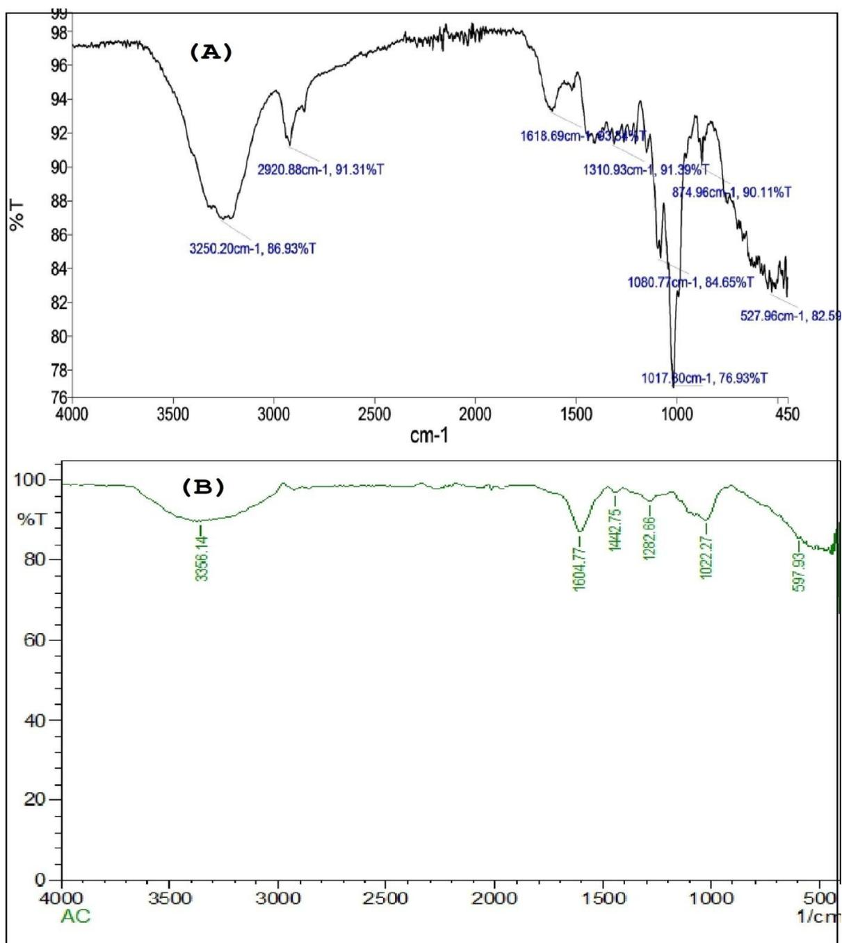
Figure 3. FT-IR spectrum of (A) Avocado (B) copper nanoparticles synthesized by avocado seed extract
