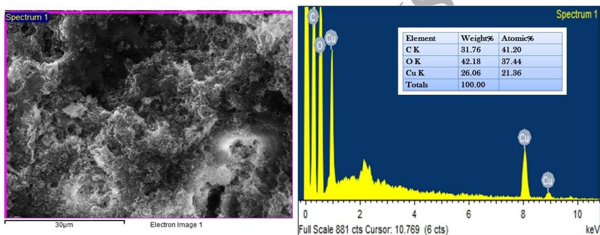
**Figure 4: EDX spectrum of Cu NPs**
