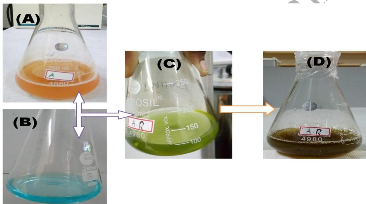
Figure 1: Visual observation of Copper nanoparticles synthesis (A) Seed extract (B) Copper sulfate solution (C) Initial color change (D) final color
