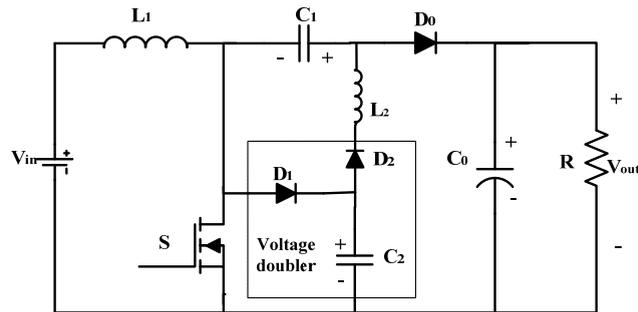
Fig. 1. Proposed converter topology circuit diagram.
