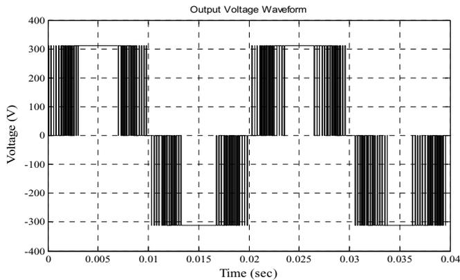
Fig. 8. Inverter output voltage waveform.
