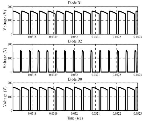
Fig. 6. The diodes voltage waveforms of the proposed converter.
