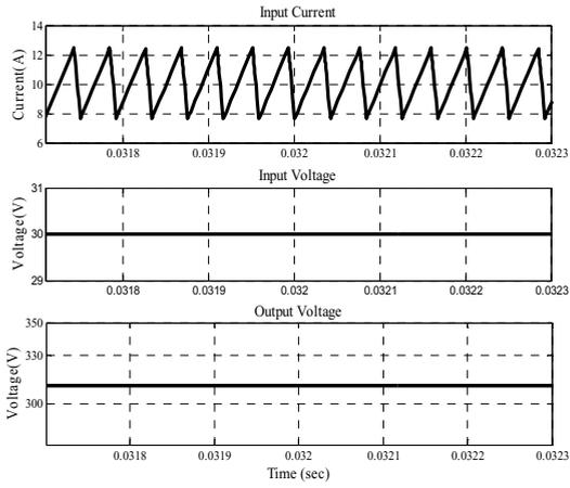
Fig. 4. The input current, voltage and output voltage waveforms.
