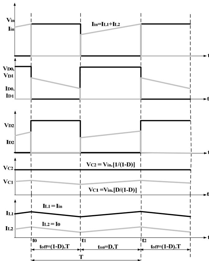
Fig. 3. Main theoretical waveforms of proposed converter at CCM operation.
