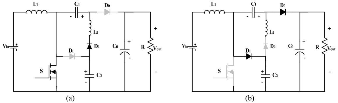
Fig. 2. Operational mode of proposed converter. a) Mode I, b) Mode II.
