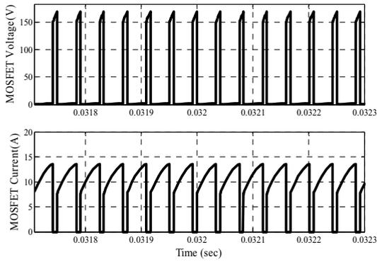
Fig. 5. The switching voltage and current waveforms.
