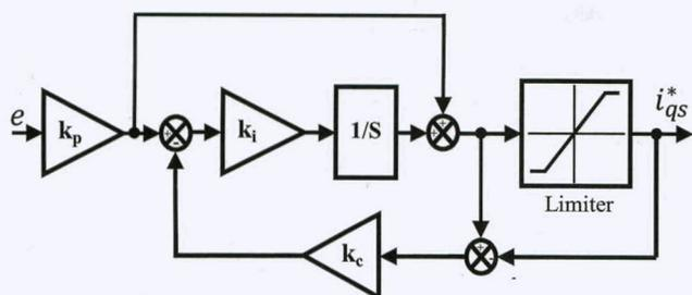
Fig. 3. Structure of PI Controller with Anti-windup.
