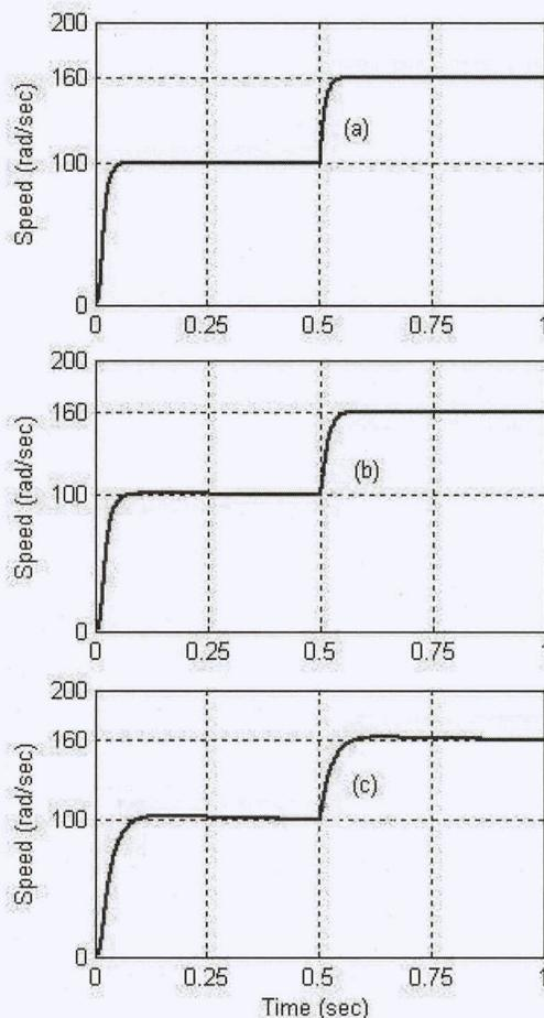
Fig. 10. Simulated speed response for a change command speed from 100 rad/sec to 160 rad/sec for (a) wavelet-fuzzy based controller (b) fuzzy controller and (c) PI controller.
