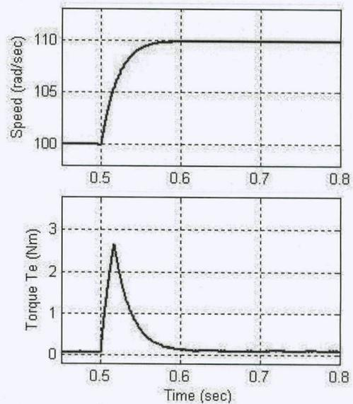
Fig.14 Simulated speed and the electromagnetic torque response of the proposed wavelet fuzzy based controller for a step speed change of 10 rad/sec at no load.
