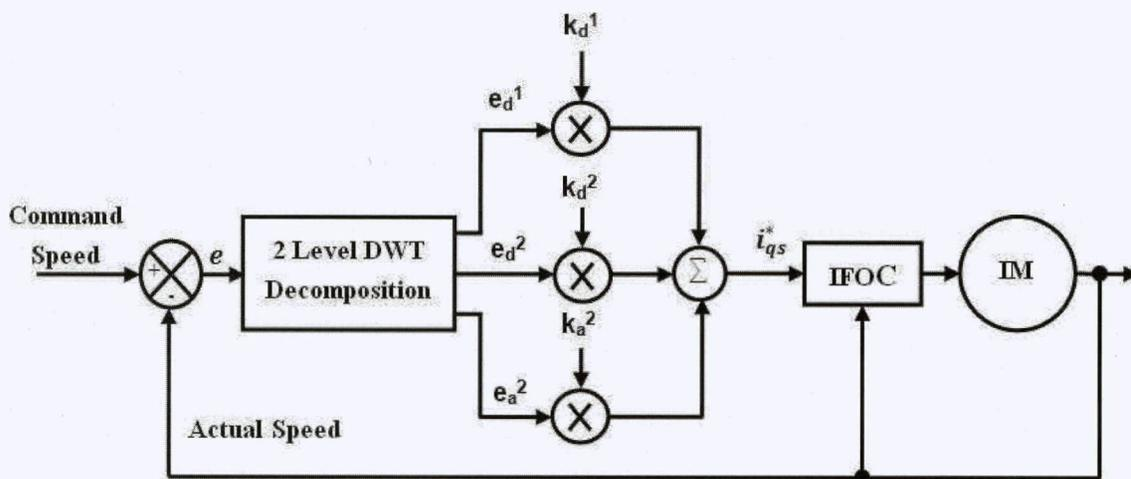
Fig. 4. Schematic of the wavelet based speed controller for IFOC of Induction motor drive
