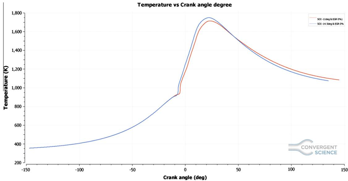
**Figure 11** In Fig 13: As the start of Injection is advanced by  $3.5^\circ$ , it makes clear that the fuel gets more time to get mixed and become more homogeneous, and hence the combustion peak temperature is higher.
