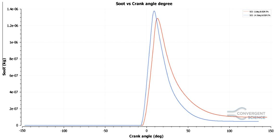
**Figure 9** Soot has decreased by 51.96%, as compared to the baseline case, at the end of the combustion. This is because early injection gives high temperatures during expansion stroke, which tends to oxidise soot particles quickly.
