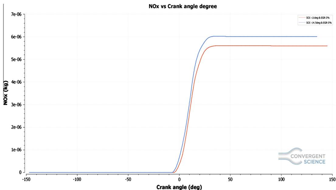
**Figure 8** From the graph (Fig. 8), it clearly indicates that  $\text{NO}_x$  has increased in improved case (Start of Injection- SOI  $14.5^\circ\text{CA}$  bTDC and EGR 0%). The  $\text{NO}_x$  content in the exhaust has been increased by 7.4%, as the SOI is advanced by  $3.5^\circ$ .
