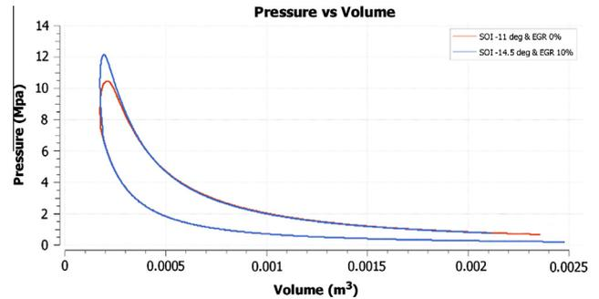
**Figure 13** Variation of in-cylinder pressure- with Volume in both baseline (red) and improved strategy (blue). In the plot, it shows that peak pressure in the second case has been increased by 0.8 MPa (which in result increases the work done).
