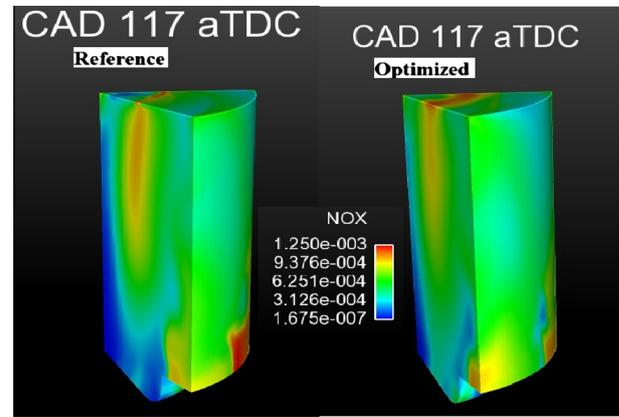
**Figure 19**  $\text{NO}_x$  content at the end of combustion in the cylinder.  $\text{NO}_x$  has been decreased by 1.2% only compared with the baseline case.
