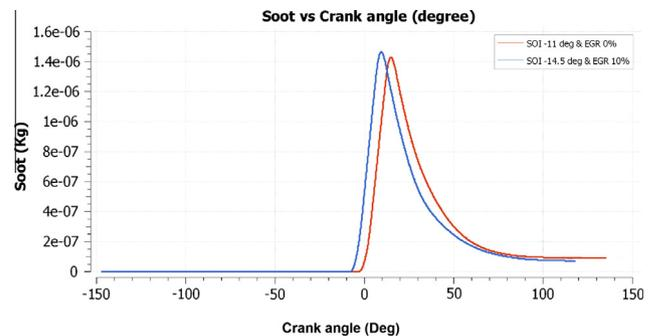
**Figure 14** Variation of soot with Crank angle in both baseline (red) and improved strategy (blue). In the above plot, it is clear that soot at the exhaust has been decreased by 21.3% compared to base-line case.
