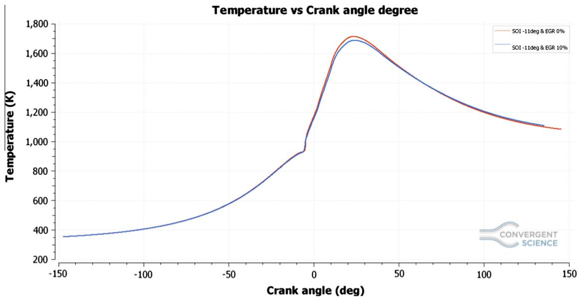
**Figure 7** Variation of in-cylinder temperature with Crank angle in both baseline (red) and improved strategy (blue). The peak temperature has been reduced due to high specific heat of  $\text{CO}_2$  present in the EGR.
