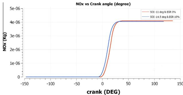
**Figure 12** Variation of  $\text{NO}_x$  with Crank angle in both base-line (red) and improved strategy (blue). The plot clearly indicates that  $\text{NO}_x$  at the end of combustion has decreased by 1.2% compared to baseline case.
