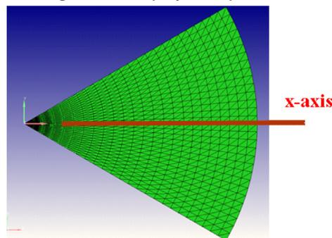
**Figure 2** A sector model geometry with the periodic boundaries appropriately symmetric about the XZ plane.
