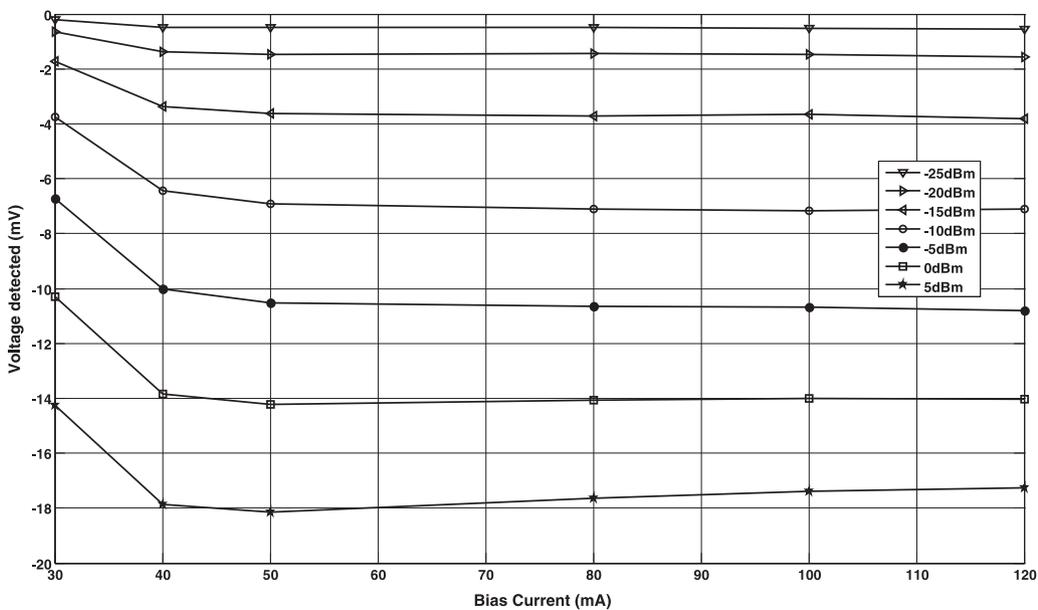
Fig. 3: Single electrode detected voltage as a function of bias currents
