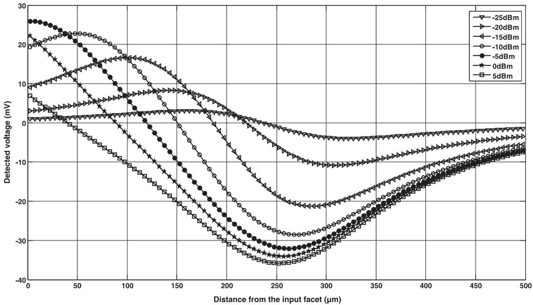
Fig. 2: Spatial variation of detected voltage for 50 mA bias current
