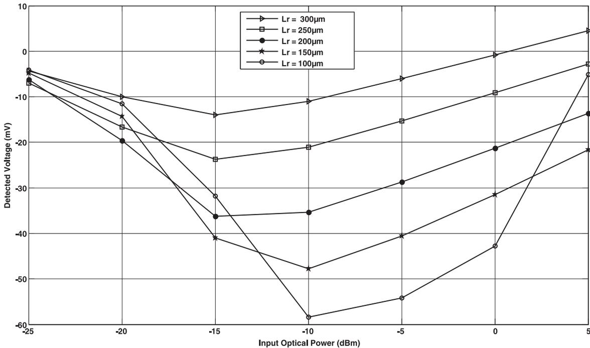
Fig. 7: Detected voltage of as a function of input optical power for different length of reference electrodes
