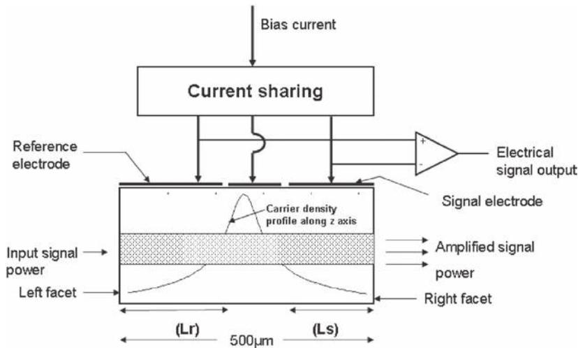
Fig. 4: Differential detection scheme
