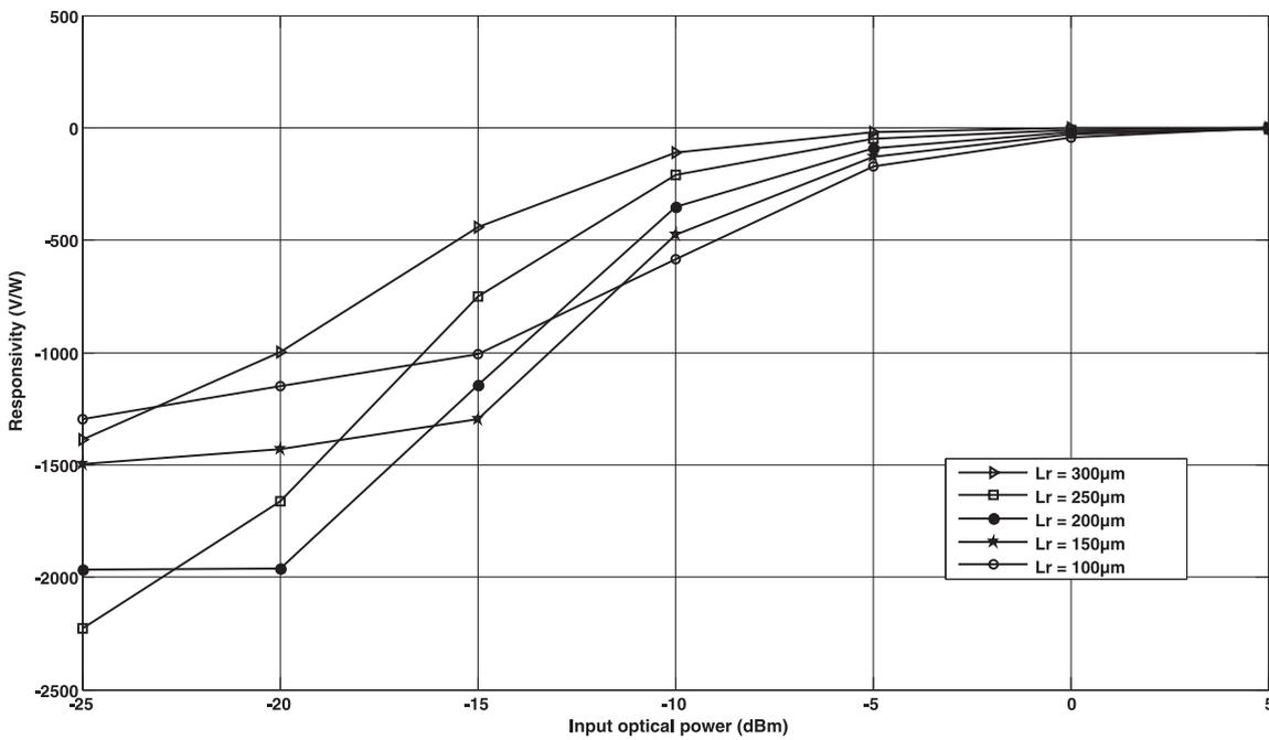
Fig. 8: Responsivity of differential detection as a function of input optical power for different lengths of reference electrode.
