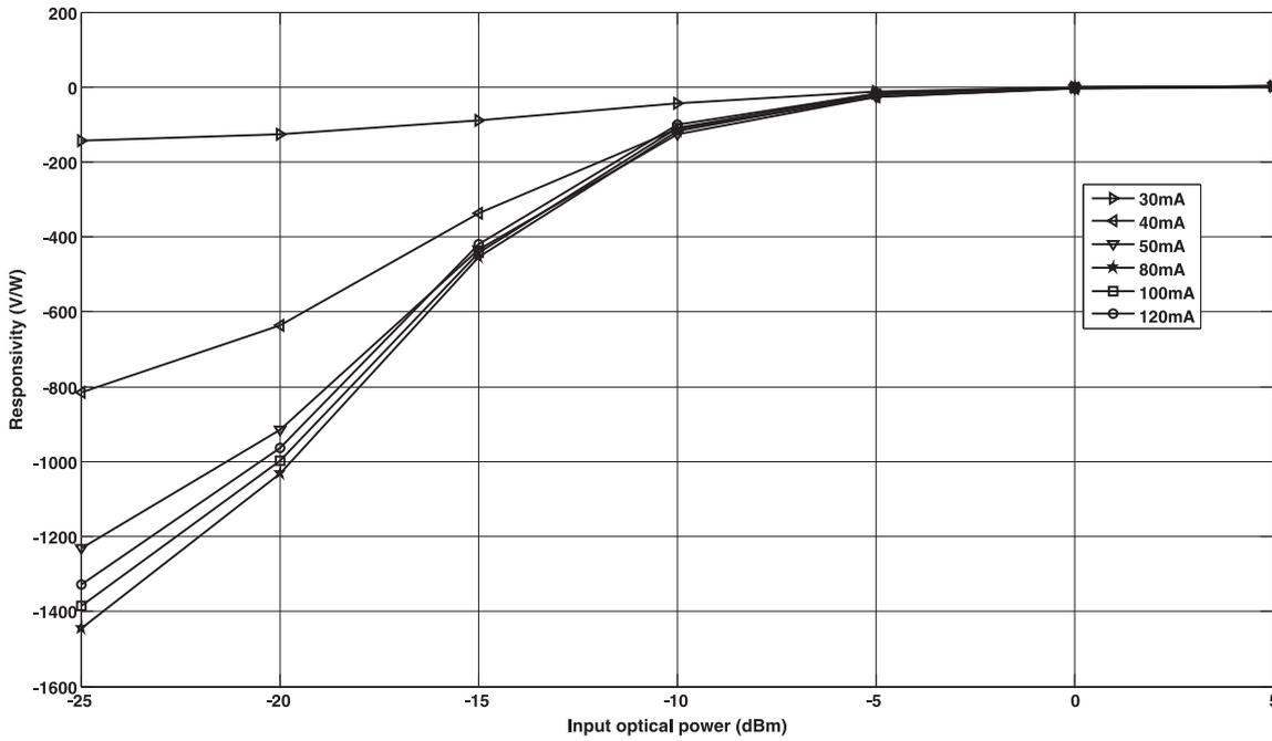
Fig. 6: Responsivity of differential detection as a function of input optical power ( $L_r = 300 \mu\text{m}$ )
