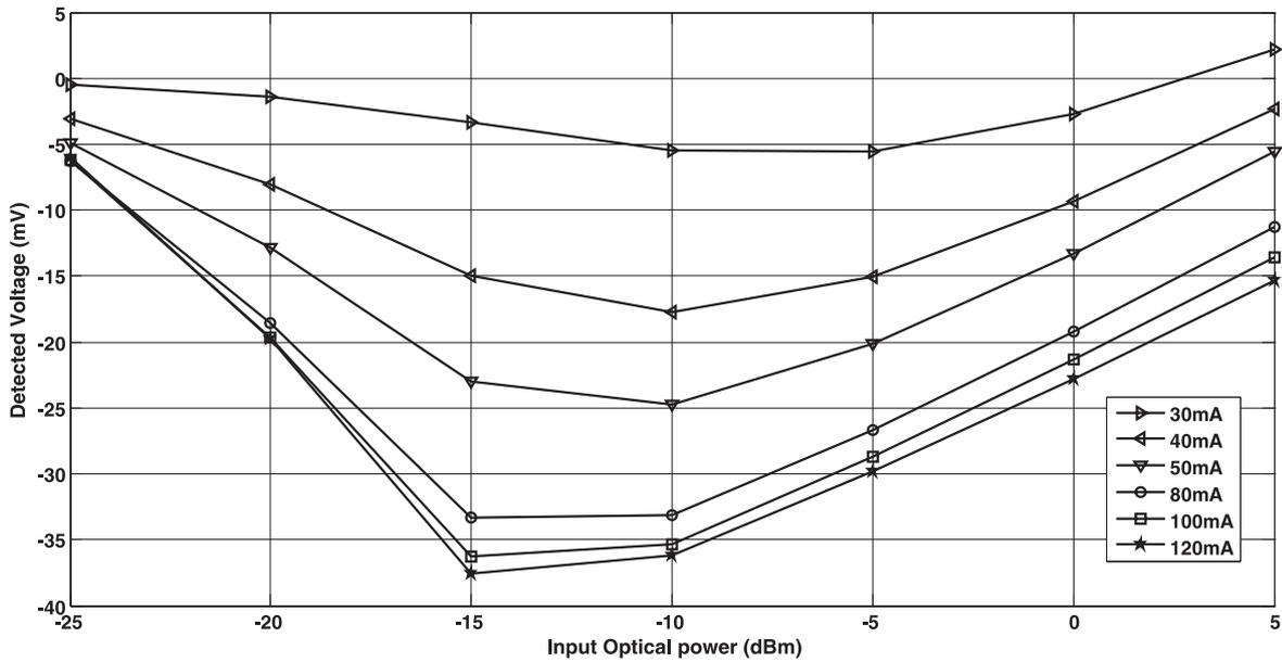
Fig. 9: Differential detected voltage for 200  $\mu\text{m}$  reference electrode length at different bias currents.
