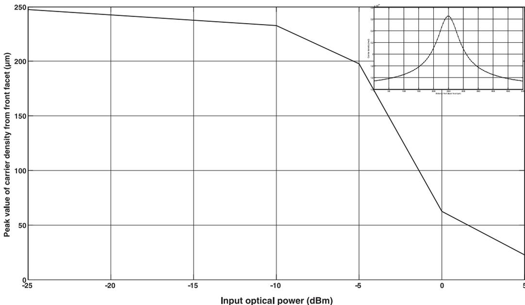
**Fig. 1:** Peak positions of the carrier density for different power levels of the TWSOA
