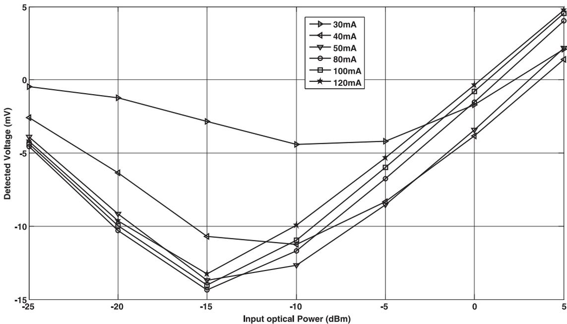
Fig. 5: Differential detected Voltage as a function of input optical power ( $L_r = 300 \mu\text{m}$ )
