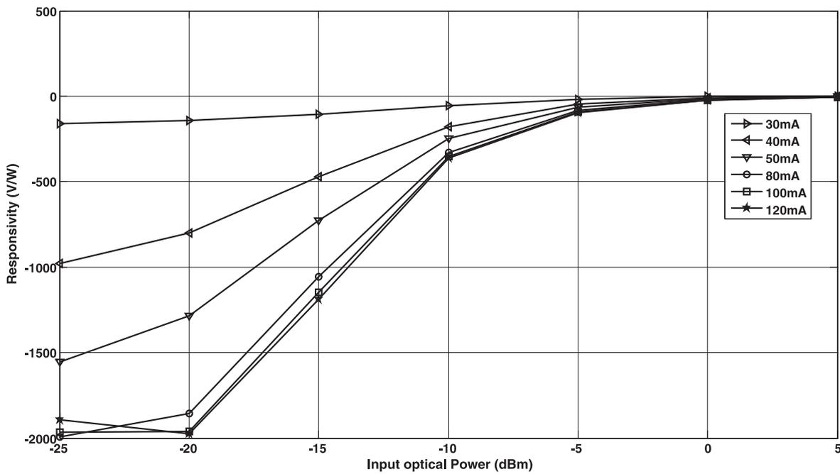
Fig. 10: Responsivity of differential detection as a function of input optical power
