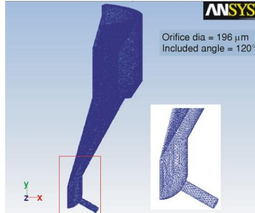
Figure 1. Mesh generated for the 120° sector of the injector (color image see our on web site)
