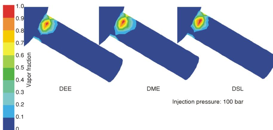
**Figure 2. Vapor fraction at injection pressure of 100 bar**
