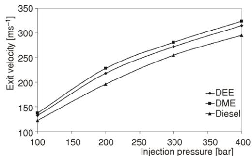
Figure 11. Variation of the exit velocity with injection pressure
