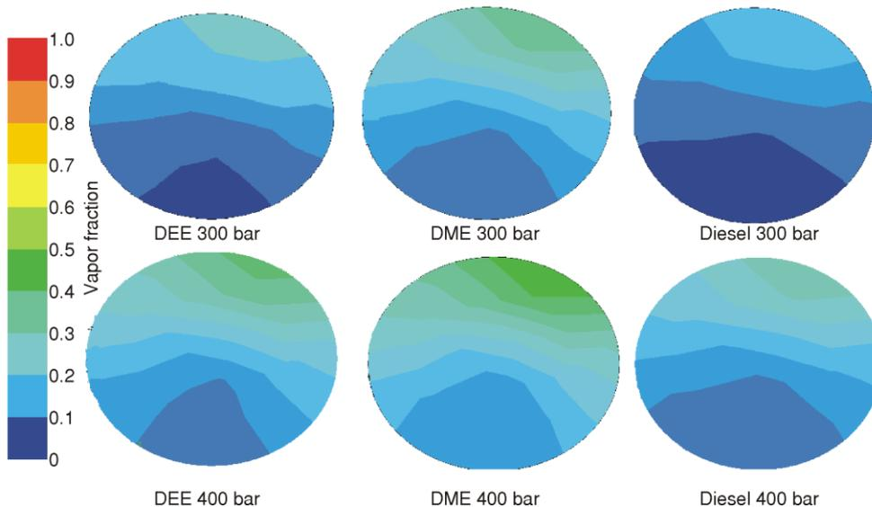
**Figure 4. Vapor fraction at the nozzle outlet for injection pressures of 300 bar and 400 bar**
