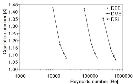
**Figure 6. Variation of cavitation number with Reynolds number**
