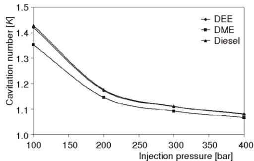
**Figure 5. Variation of cavitation number with injection pressures**
