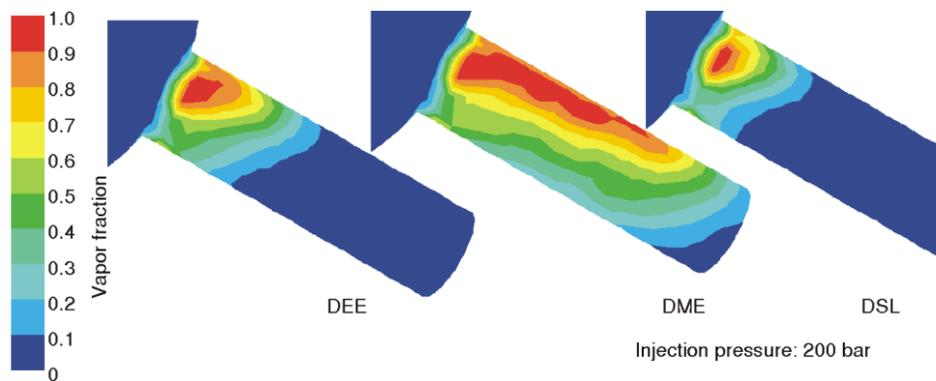
**Figure 3. Vapor fraction at injection pressure of 200 bar**
