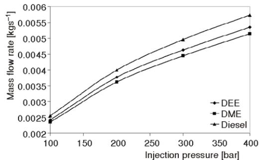
Figure 12. Variation of the mass flow rate with injection pressure
