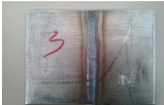
Fig.1. Sample piece welded using TIG welding with 2.0 mm root gap
