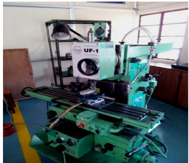
**Fig. 3** Knee-type vertical milling machine
