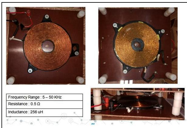
Figure 16. Hardware image of the transmitting and receiving coils.
