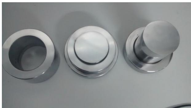
**Figure 1.** Die used for target preparation.
