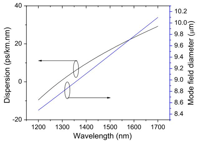
Fig. 7. (Color online) Spectral variations of the dispersion and the mode-field diameter of optimized BIF.
