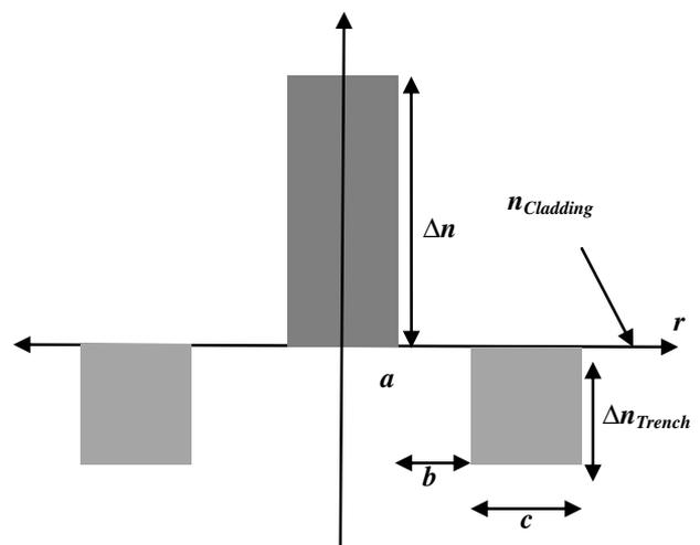
Fig. 1. Bend-insensitive optical fiber (BIF).
