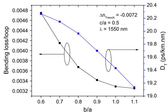
Fig. 4. (Color online) Effects of trench separation on the bending loss and dispersion characteristics. Bending loss was determined at the loop diameter of 5 mm.
