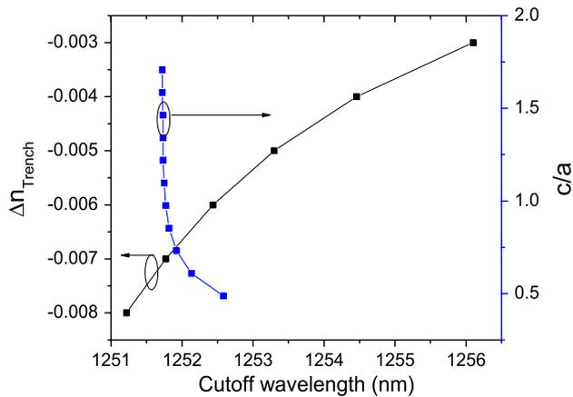
Fig. 2. (Color online) Effects of trench index difference and trench width on the cutoff wavelength.
