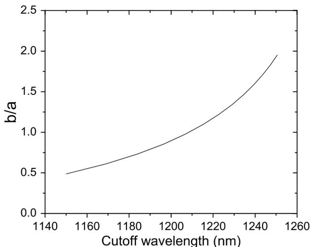
Fig. 3. Effects of trench separation on the cutoff wavelength.
