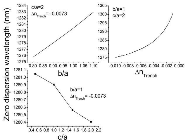
Fig. 8. Dependence of zero dispersion wavelength on trench parameters.
