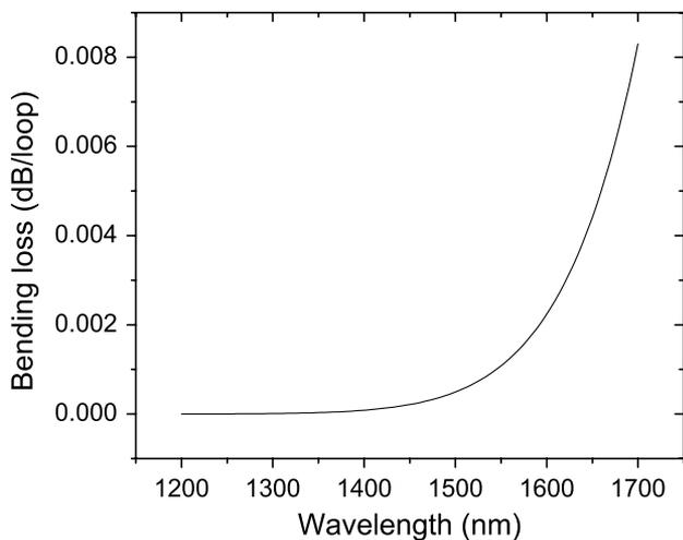
Fig. 6. Spectral variation of the bending loss of optimized BIF.
