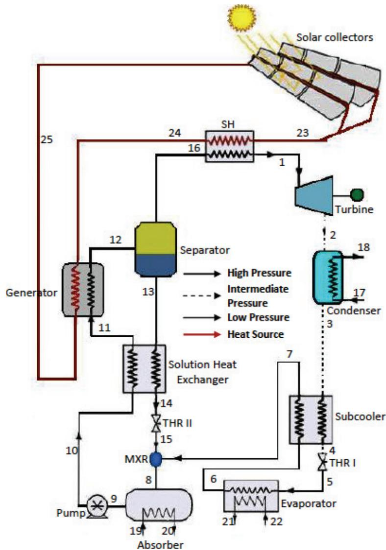
Fig.1 Schematic layout of common (LiBr-water and aqua-ammonia) cooling cogeneration cycle.
