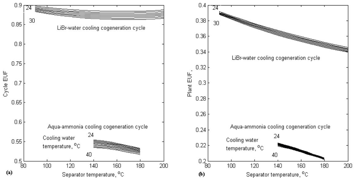
Fig. 3. (a) Cycle Energy Utilization Factor and (b) Plant Energy Utilization Factor of the cooling cogeneration cycle.
