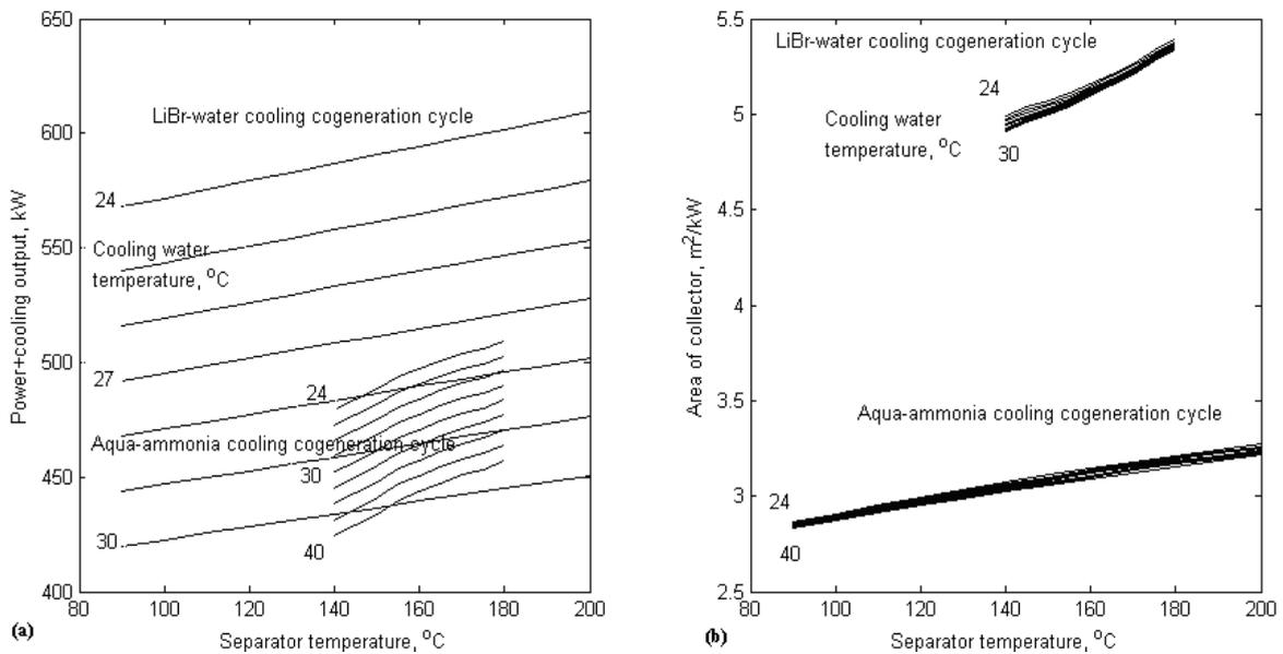
Fig.4 Comparisons of aqua-ammonia and LiBr-water cooling cogeneration cycle on (a) power+cooling output and (b) area of collector.
