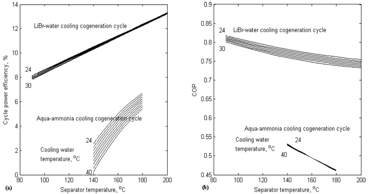
Fig. 2. Performance of (a). Cycle power efficiency and (b). COP of cooling cogeneration cycle
