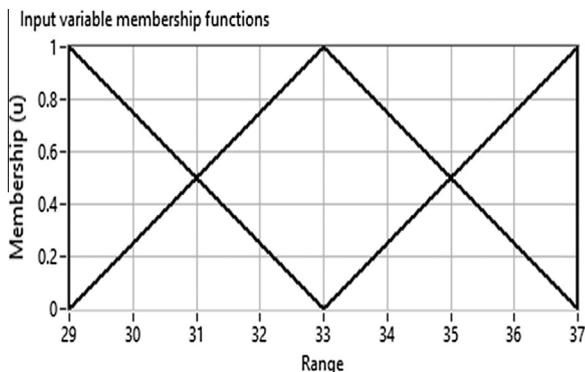
**Figure 4** Membership function for the crystalline size.
