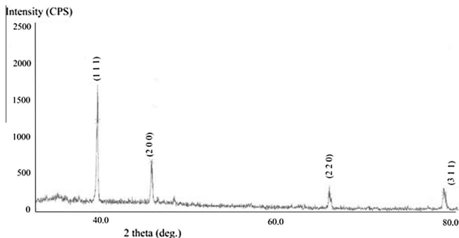
Figure 15 HCS chip XRD image of experiment 12.
