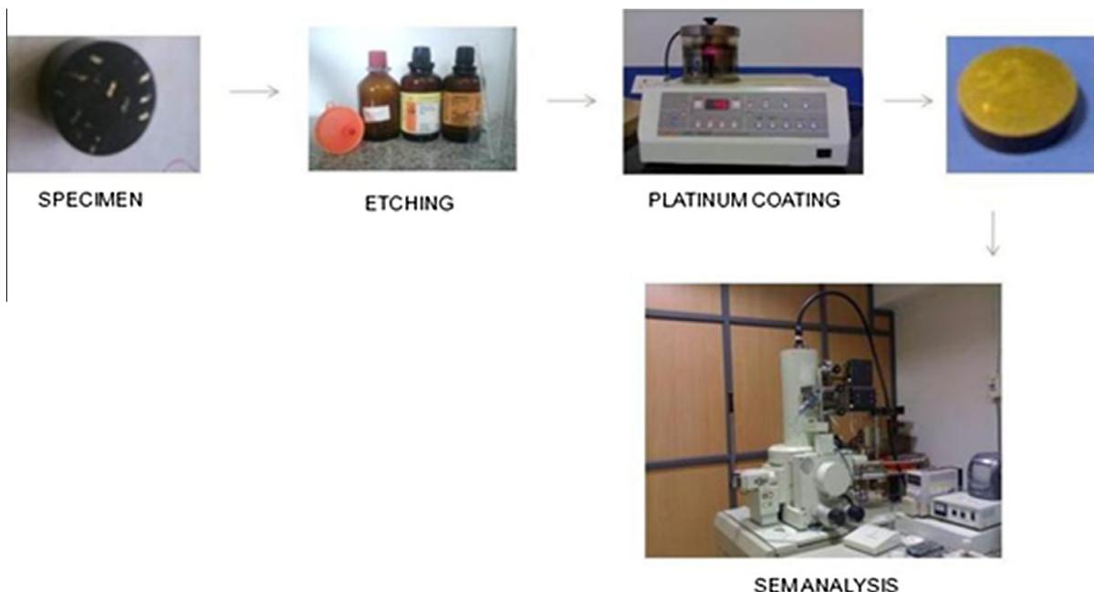
Figure 2 FEG-SEM – flow diagram.
