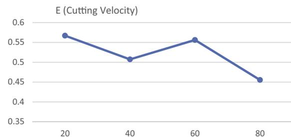
**Figure 10** MRPI response graph for cutting velocity.
