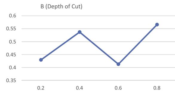
**Figure 7** MRPI response graph for depth of cut.
