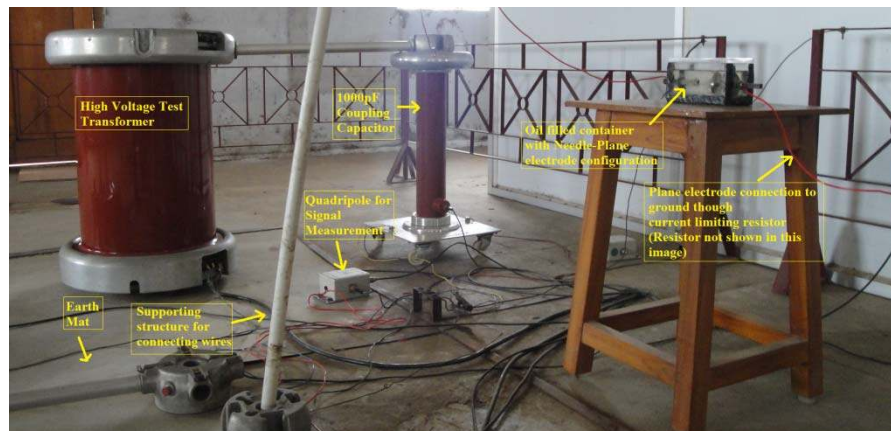
Figure 2. Setup for PD stressing experiment
