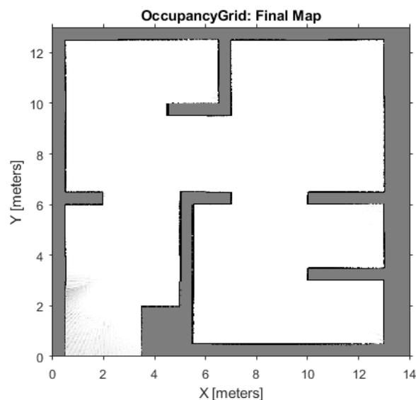
**Fig. 5.** Binary occupancy grid generated by LIDAR simulation.
