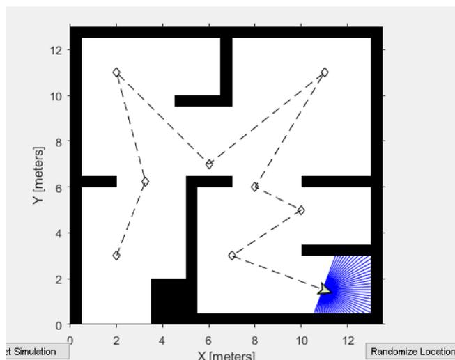
**Fig. 4.** Path generation using LIDAR simulation. (in MATLAB).
