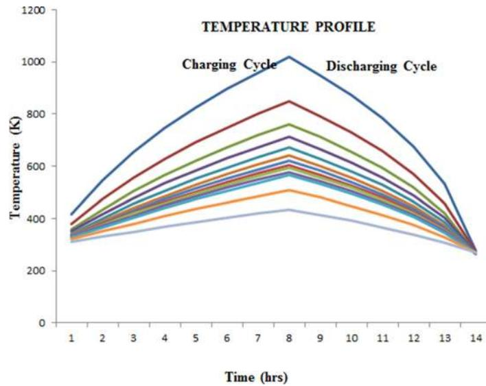
FIG. 8. Temperature profile for different tank volumes.
