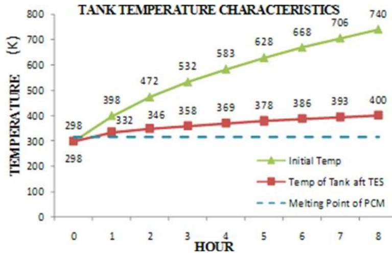
FIG. 17. Tank temperature for CAES-AA on an hourly based simulation during charging.
