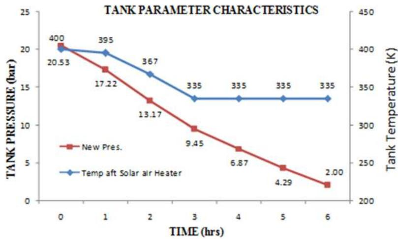
FIG. 20. Tank parameter for CAES-AA-solar on an hourly based simulation during the discharging cycle.
