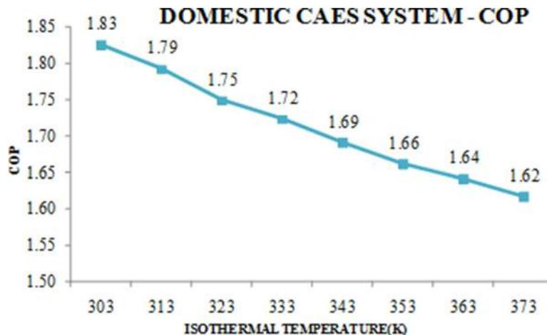
FIG. 15. Coefficient of performance for small scale CAES.
