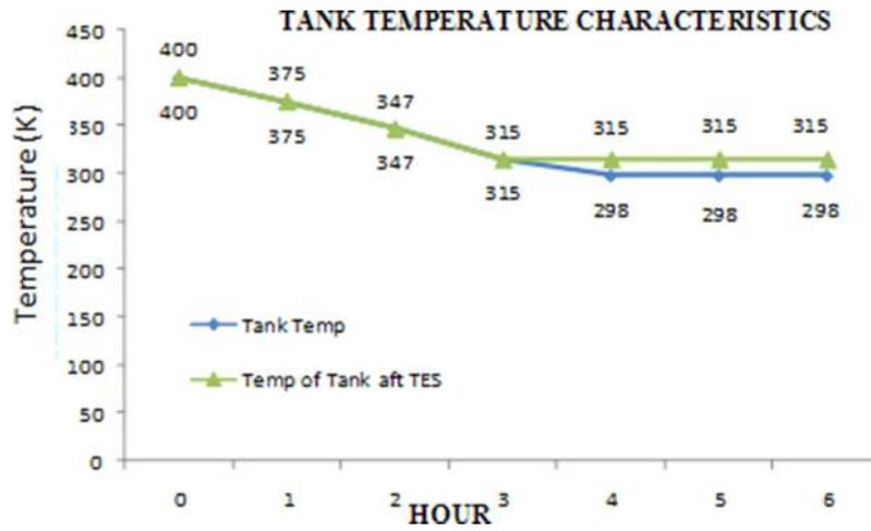
FIG. 19. Tank temperature for CAES-AA on an hourly based simulation during discharging.
