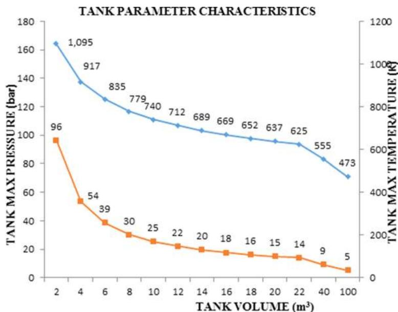
FIG. 7. Tank parametric variations for different ranges of tank volume.
