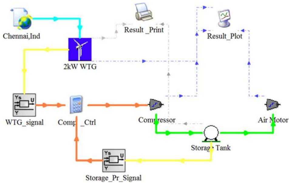
FIG. 4. Schematic layout of the CAES system in the TRNSYS V17 platform.
