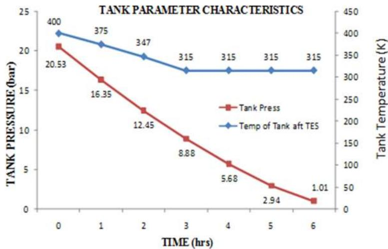
FIG. 18. Tank parameter for CAES-AA on an hourly based simulation during discharging.
