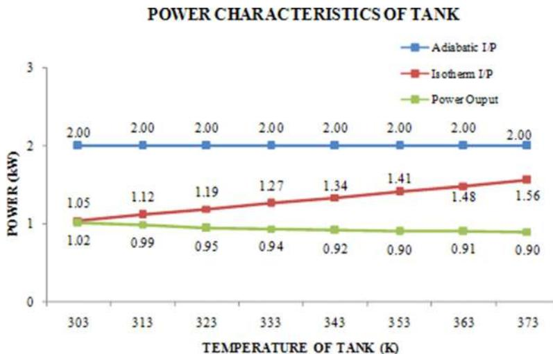
FIG. 11. Power characteristics of the CAES tank in an isothermal condition.
