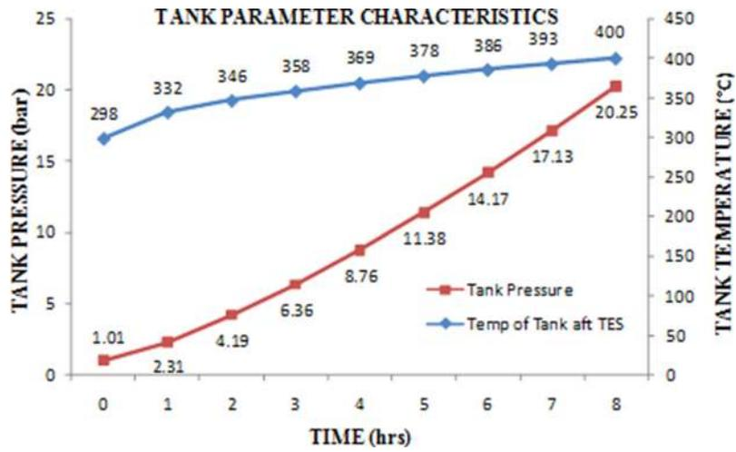
FIG. 16. Tank parameter for CAES-AA on an hourly based simulation during charging.
