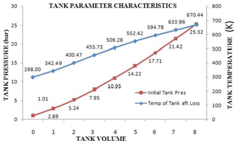
FIG. 9. Hourly parametric characteristics for the charging cycle.
