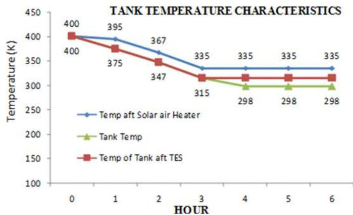
FIG. 21. Tank temperature for CAES-AA-solar on an hourly based simulation during the discharging cycle.
