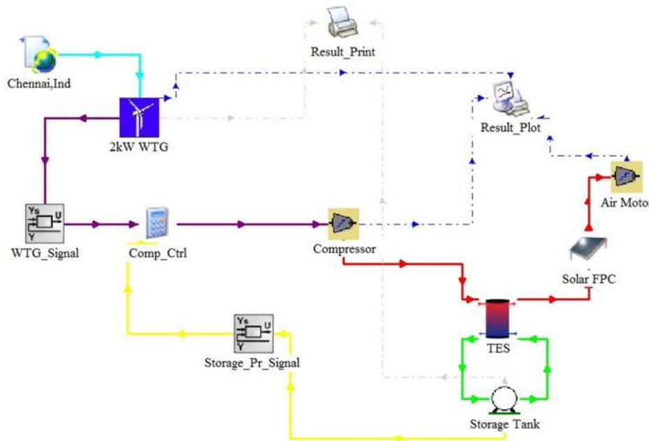
FIG. 6. Schematic layout of the CAES-AA-solar system in the TRNSYS V17 platform.
