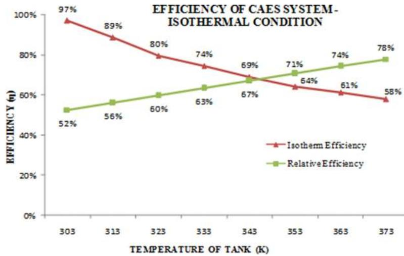
FIG. 12. Efficiency of the CAES system—isothermal condition.
