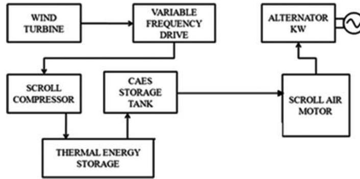
FIG. 2. Block diagram of the advanced adiabatic CAES system with TES.
