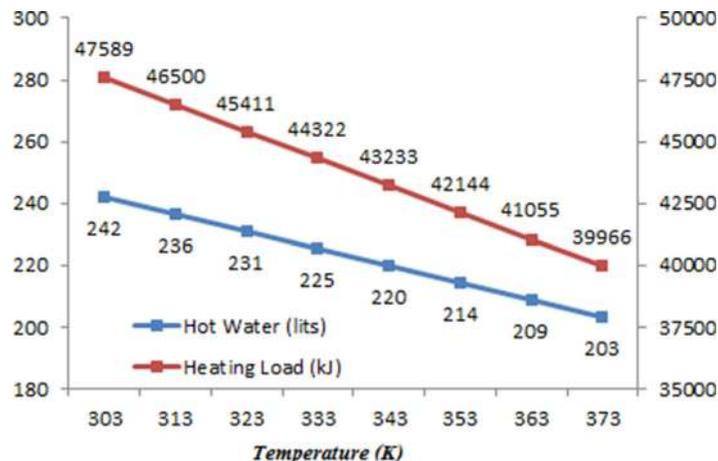
FIG. 13. Heating load calculation and hot water production from the CAES system.
