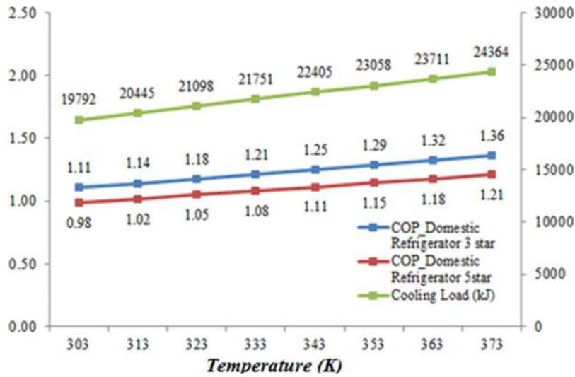
FIG. 14. Cooling load calculation and comparative electric load for a refrigerator.
