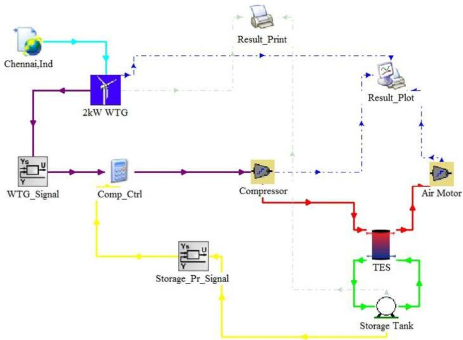
FIG. 5. Schematic layout of the CAES-AA system in the TRNSYS V17 platform.
