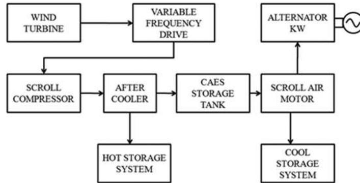
FIG. 1. Block diagram of the proposed system—poly-generation.
