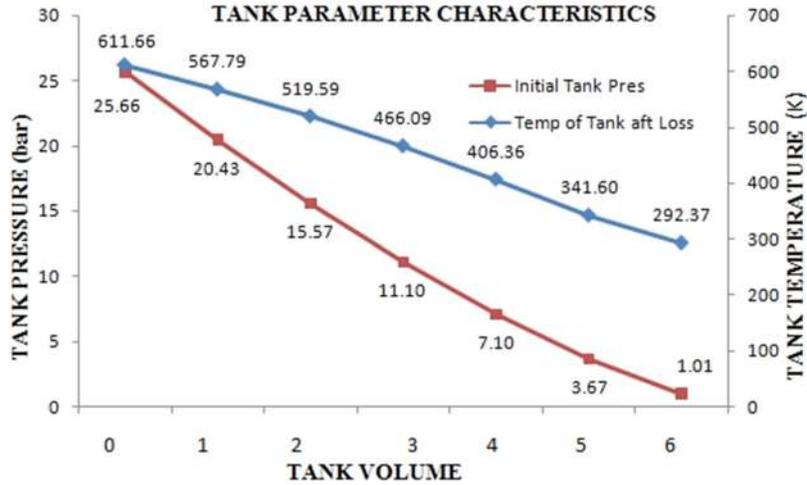
FIG. 10. Hourly parametric characteristics of the discharging cycle.
