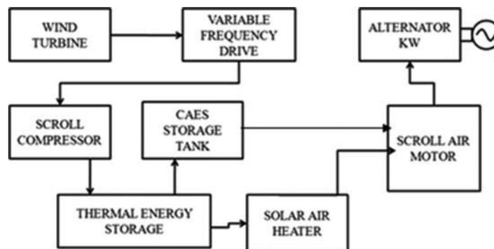
FIG. 3. Block diagram of the solar integrated advanced adiabatic CAES system with TES.
