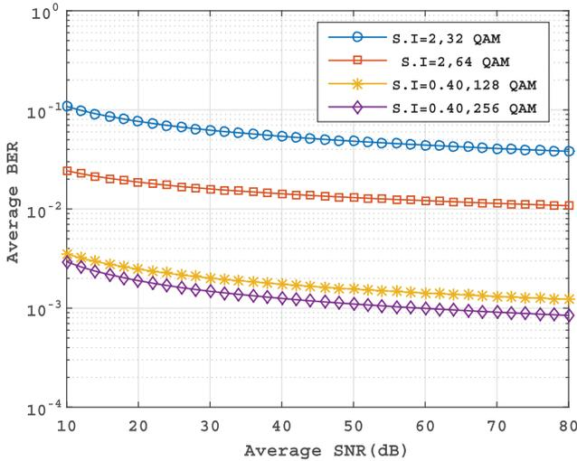
**Figure 4:** BER performance versus SNR for varying QAM modulation order.
