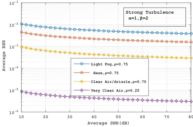
Figure 6: BER versus SNR for various weather conditions for the strong turbulence condition.
