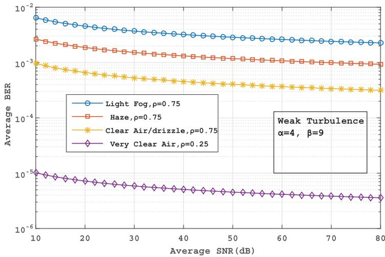
Figure 7: BER performance versus SNR for different weather conditions for the weak turbulence.
