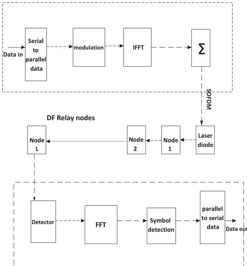
Figure 2: Schematic of Multi-hop DF FSO system.
