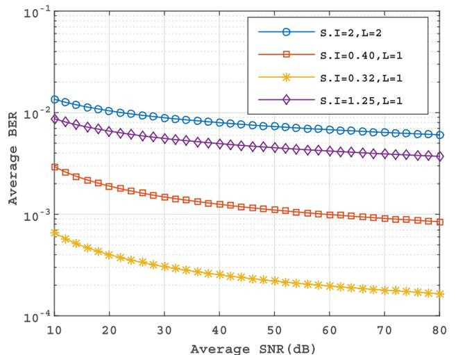
Figure 3: BER performance versus SNR for different S.I. and relays.
