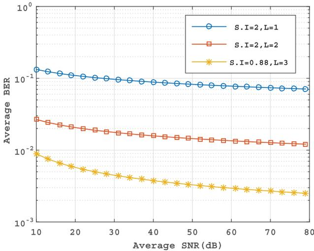
**Figure 5:** BER performance versus SNR for different number of relays.
