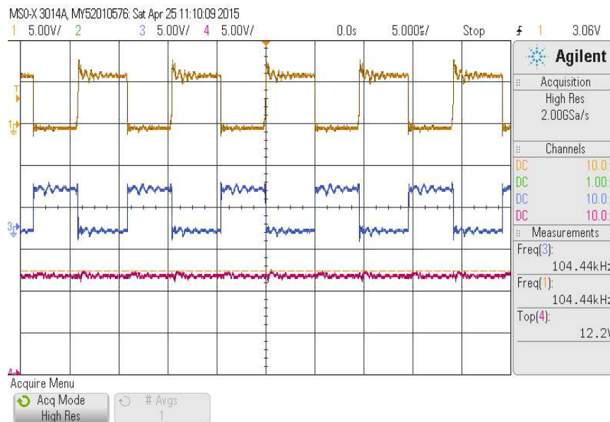
Figure 18. Output voltage for subtraction circuit
