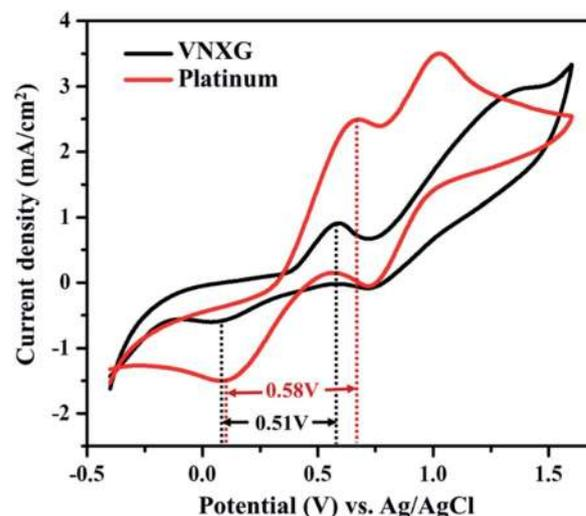
Fig. 7 Cyclic voltammogram of the VN<sub>x</sub>G and Pt electrode at a scan rate of 50 mV s<sup>-1</sup> vs. Ag/AgCl.
