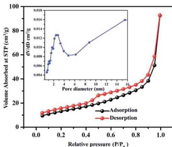
Fig. 6 BET adsorption-desorption isotherm of the VN<sub>x</sub>G (inset: BJH pore size distribution obtained for VN<sub>x</sub>G).
