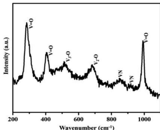
Fig. 3 Raman spectroscopy analysis of VN<sub>x</sub>G.
