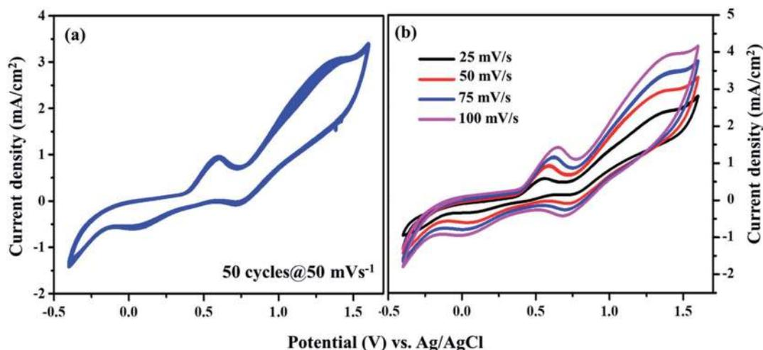
Fig. 8 (a) Cyclic voltammogram of the VNXXG tested for the 50-cycle stability study at a scan rate of  $50 \text{ mV s}^{-1}$  and (b) CV at different scan rates vs. Ag/AgCl.
