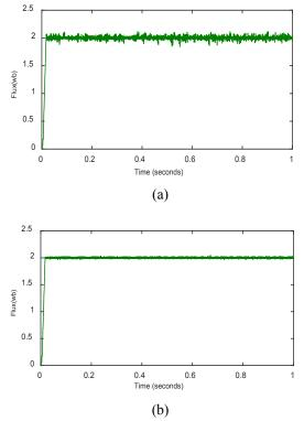
**Figure 9.** Stator flux (reference flux =2) at 2 KHz (a) and 5 KHz (b) switching frequency.
