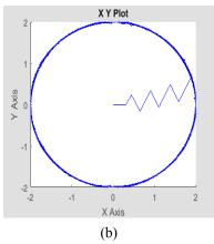
**Figure 10.** Flux trajectory at 2 KHz (a) and 5 KHz (b) switching frequency.
