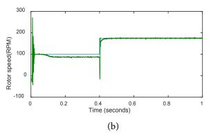
**Figure 8.** Rotor speed at 2 KHz (a) and 5 KHz (b) switching frequency.
