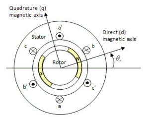
Figure 2. PMSM in D-q axes reference frame.
