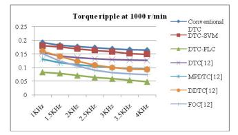
**Figure 14.** Analysis of Electromagnetic torque ripple at 1000 r/min for the proposed and existing control techniques implemented in<sup>12</sup> at different frequencies.
