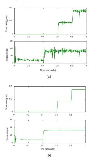
**Figure 11.** Pump output at 2 KHz (a) and 5 KHz (b) switching frequency.
