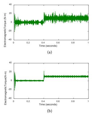
**Figure 7.** Electromagnetic torque at 2 KHz (a) and 5 KHz (b) switching frequency.
