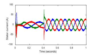
**Figure 6.** Stator current at 2 KHz (a) and 5 KHz (b) switching frequency.
