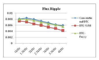
**Figure 12.** Analysis of Stator flux ripple at 500 r/min of three control techniques at different frequencies.
