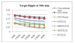
**Figure 13.** Analysis of Electromagnetic torque ripple at 500 r/min for proposed and existing control technique implemented in<sup>12</sup> at different frequencies.
