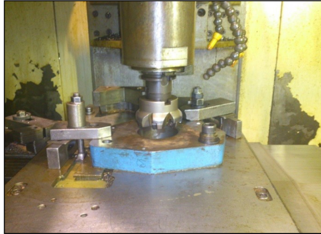
Fig. 1 Tie bar plate located in the machining set up
