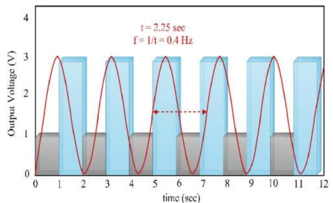
**FIGURE 8** Output voltage observed in the developed PEHS
