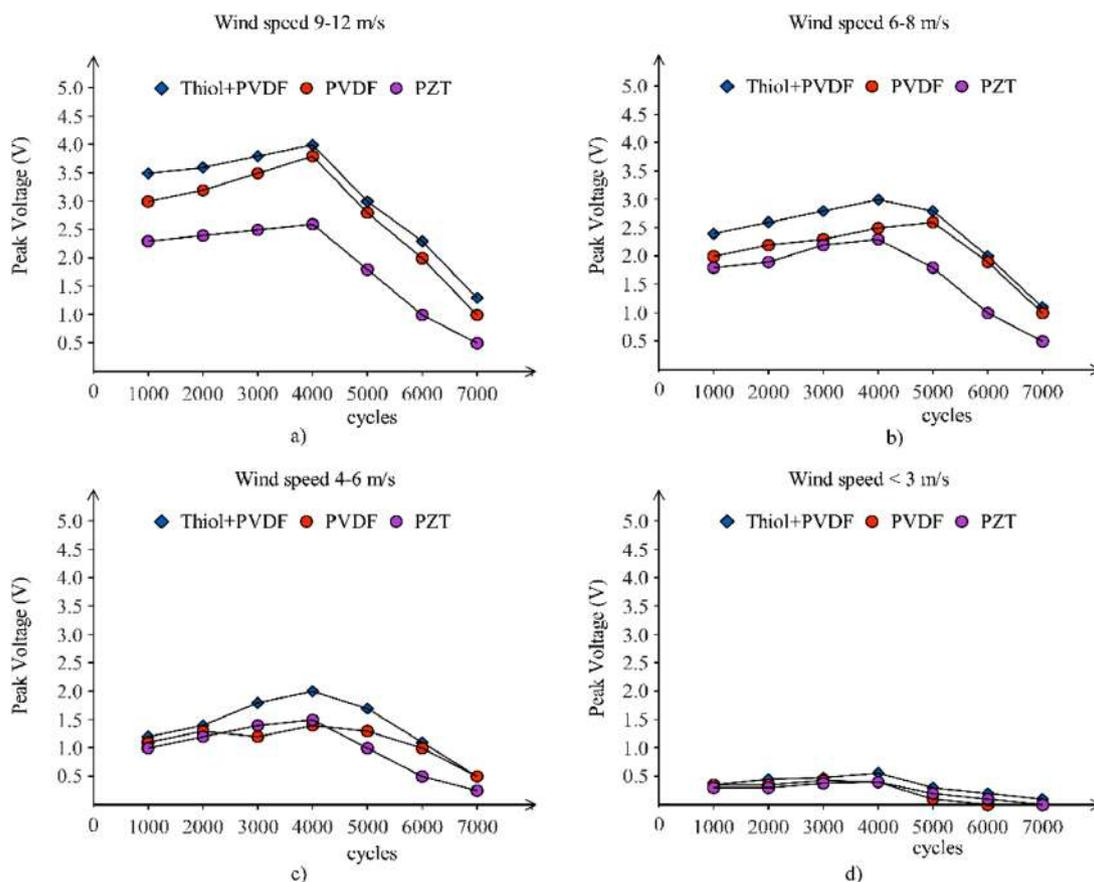
FIGURE 10 Peak voltage observed in the studied PEHS
