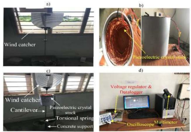
FIGURE 4 Experimental setup of the fabricated PEHS
