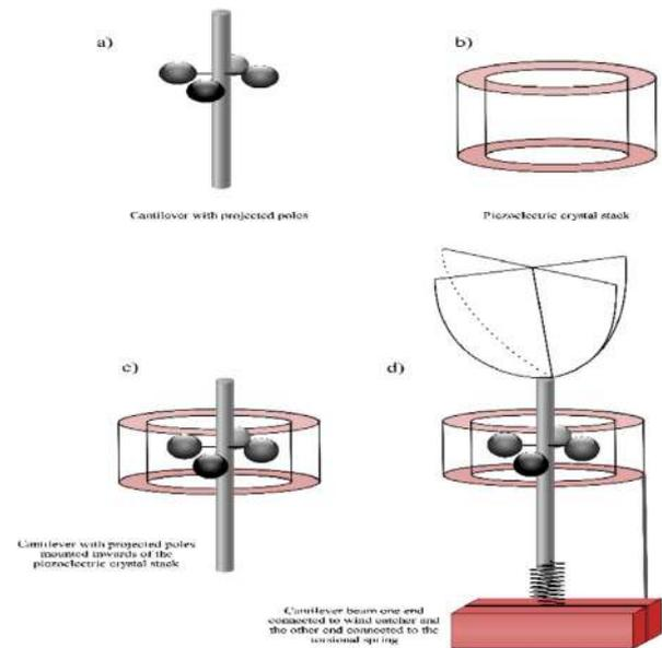
**FIGURE 1** Modelling of the proposed PEHS, (a) cantilever with projected poles, (b) piezoelectric crystal stack, (c) piezoelectric crystal stack fixed to cantilever, (d) complete setup of proposed PEHS
