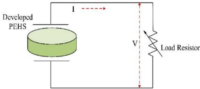
**FIGURE 5** Circuit diagram from the load test
