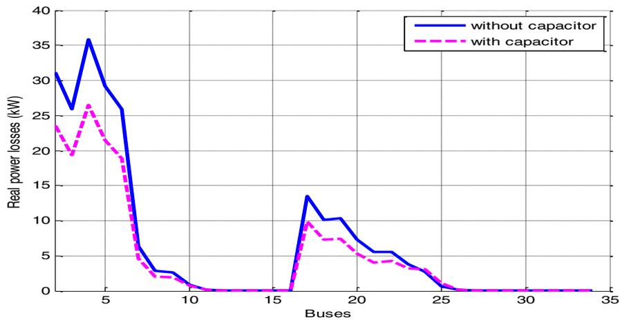
Fig. 4. Real power line losses of IEEE 34-bus radial distribution system.
