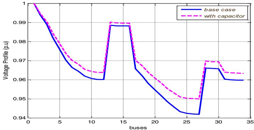
Fig. 3. Voltage profile of the IEEE 34-bus system with and without capacitor
