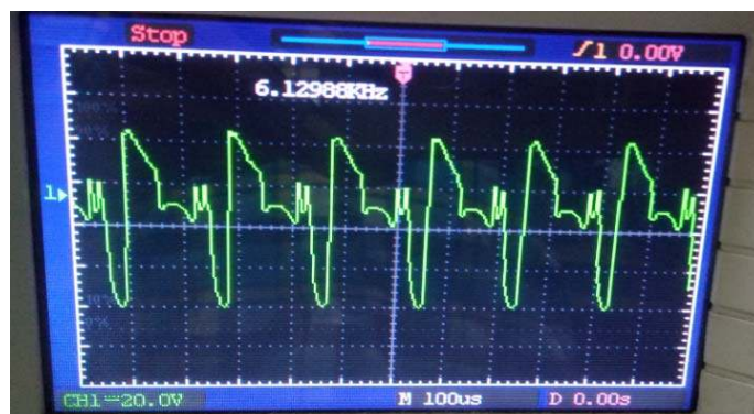
Fig. 6.5. Voltage response of inverter
