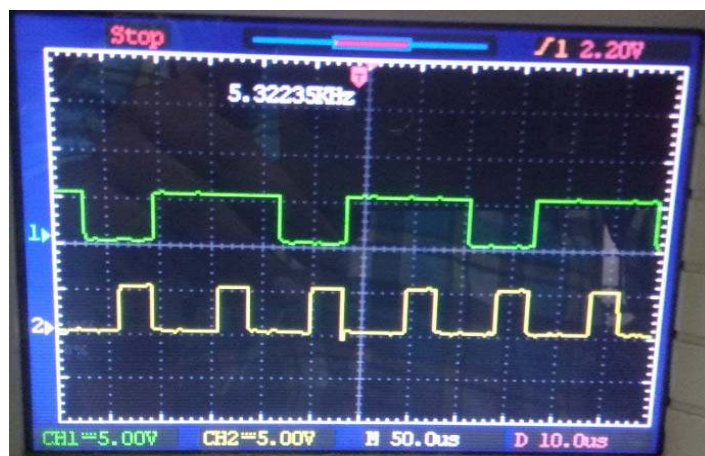
Fig. 6.4. Switching Pulses for M1 and M2
