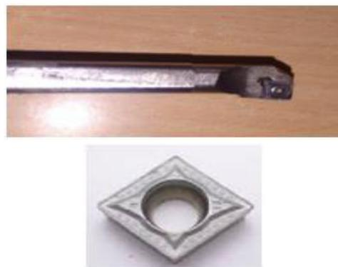
Figure 3. Carbide insert and carbide insert with tool holder.
