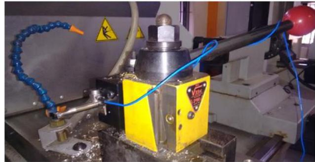
Figure 2. Arrangement of sensor on the boring bar.
