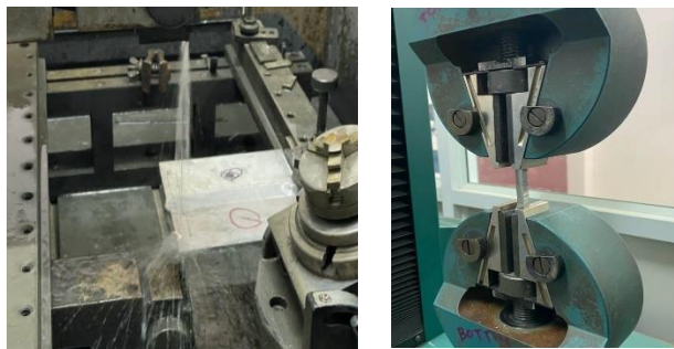
Figure 3. Tensile specimen prepared using wire-cut EDM and UTS machine arrangement for tensile tests.
