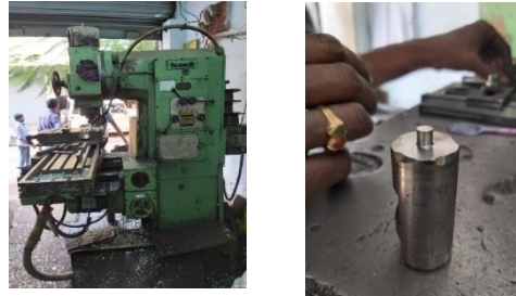
Figure 1. Lathe machine and the tool used for friction stir processing.
