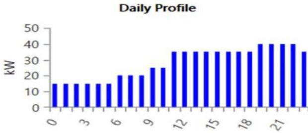
FIGURE 6. Daily load profile of load data.
