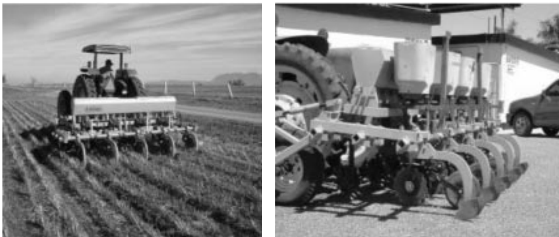
Figure 12. Left-Multi-crop/multi-use implement configure for reshaping permanent beds and applying basal fertilizer; Right-Same implement configured for bed reshaping, fertilizing and maize planting.
