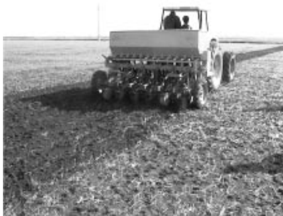
Figure 5. Photo of the Moroccan seed drill operating at farmer's field in the first year introduction of the no till system. The drill is operating on dry soil with high percent of stones and no residue on the soil surface. (El gharras et al., 2004)
