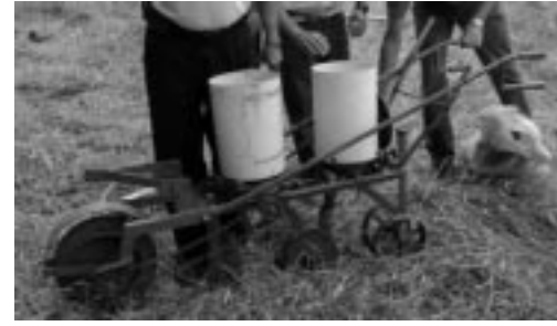
Figure 12. The Gralha azul animal traction no-till planter and fertiliser applicator developed at IAPAR in the mid-1980s
