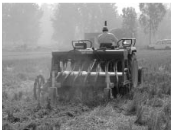
Figure 3. New prototype of Happy Seeder in operation with 35 HP tractor
