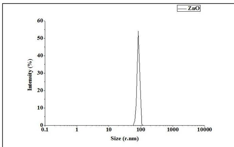
**Figure 1: Particle Size Analyser for ZnO nanocatalyst**
