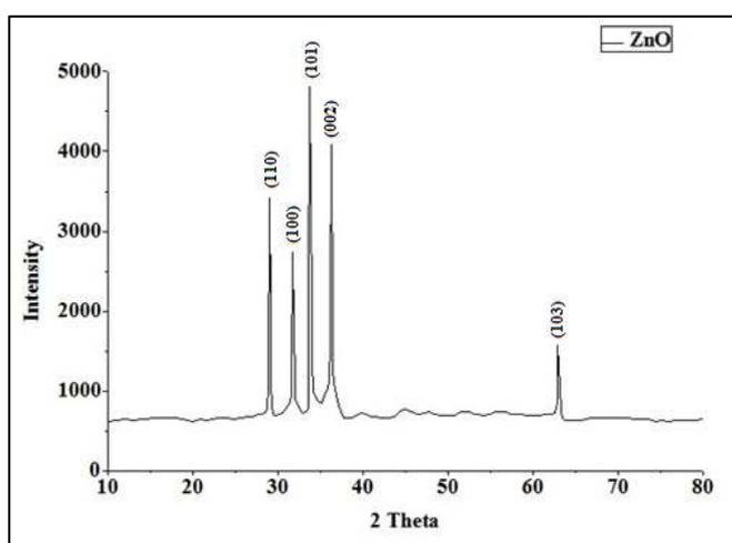
**Figure 2: XRD Patterns for ZnO**
