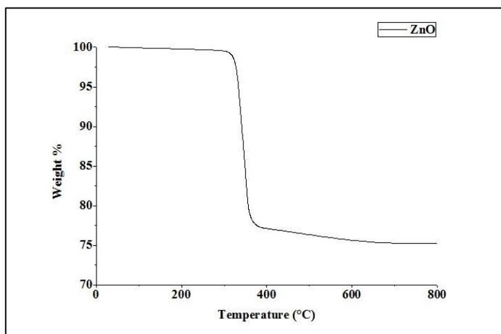
**Figure 3: TGA Plot for ZnO**
