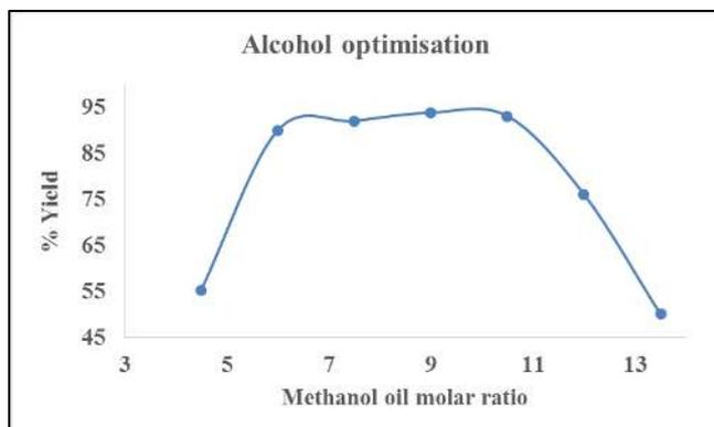
**Figure 7: Effect of methanol oil molar ratio**
