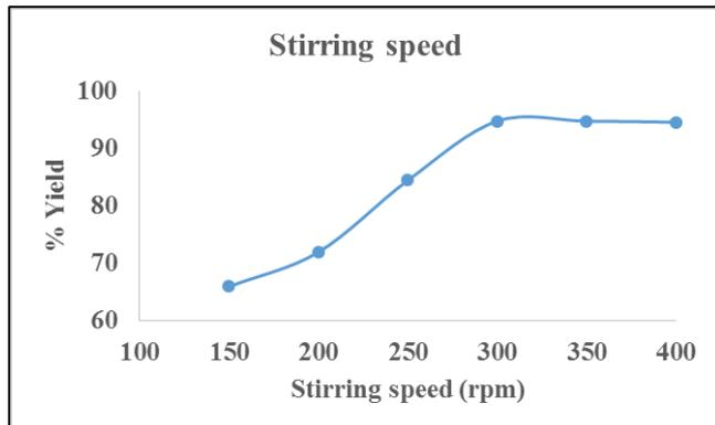
**Figure 8: Effect of stirring speed**
