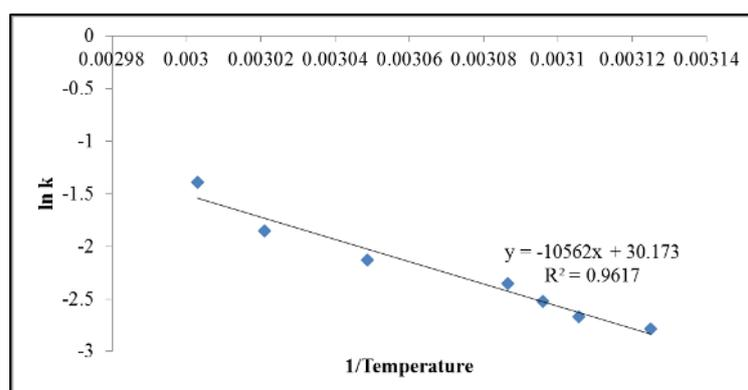
**Figure 10: A linear graph of Arrhenius equation ( $\ln k$  v/s  $1/T$ )**
