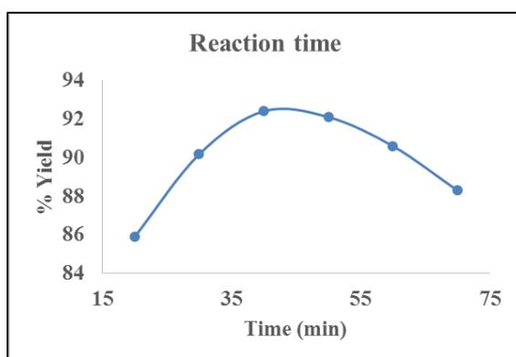
**Figure 6: Effect of reaction time**
