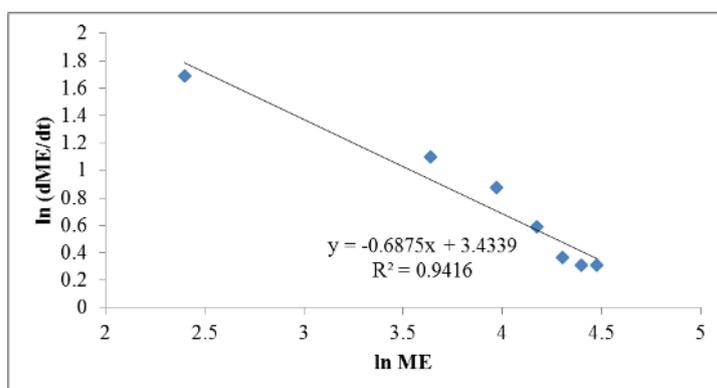
**Figure 9: A linear graph reaction rate vs yield on logarithmic graph (%) for transesterification of dairy waste scum oil.**
