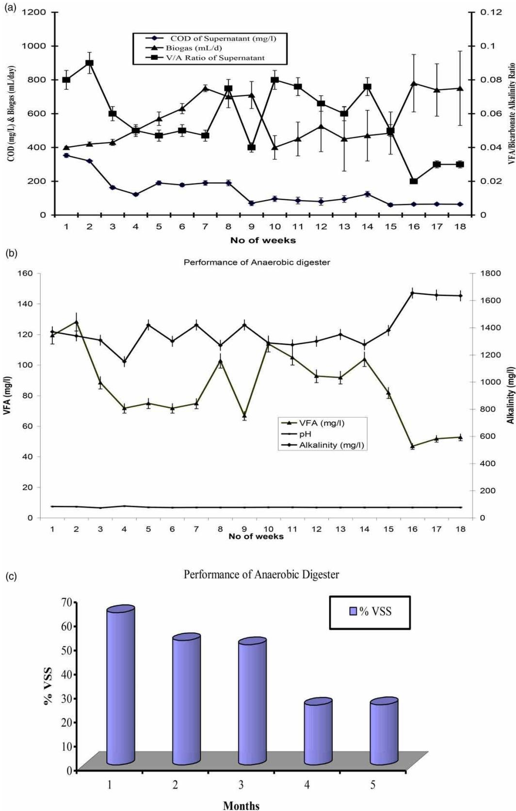
**Figure 2** | Performance during operation of an anaerobic digester. (a) Profile of Biogas production, COD and ratio of VFA/bicarbonate alkalinity (V/A) of digester effluent. (b) Profile of VFA, pH and alkalinity in the digester. (c) Profile of percentage VSS in the digester with time of operation.
