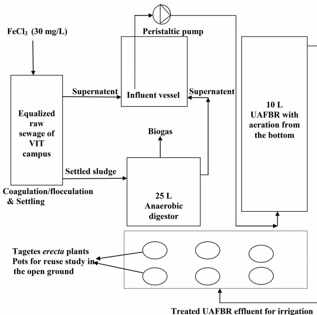
**Figure 1** | The schematic of the lab-scale decentralized wastewater treatment system.
