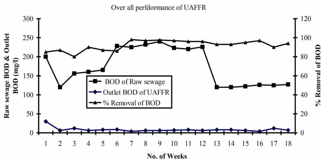
Figure 3 | Performance of UAFBR operation in BOD removal. (UAFBR in figure denotes UAFBR).
