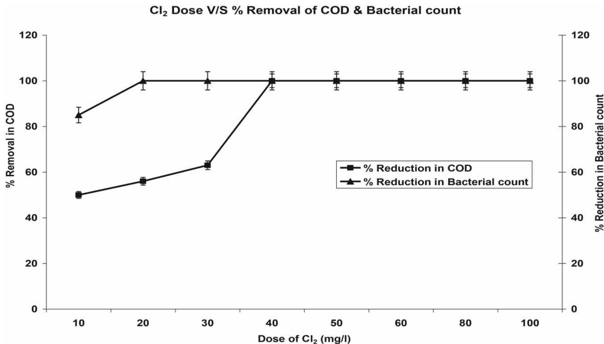
**Figure 4** | Results of chlorination of UAFBR effluent.
