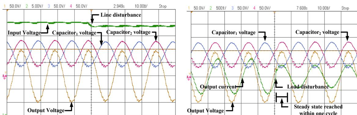
Fig. 2. (a) Line Regulation; (b) Load Regulation.
