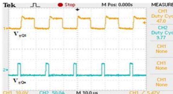
**Fig. 9:** Waveforms of Gate Pulses for the Switches  $Q_1$  and  $Q_a$  in Boost Mode.
