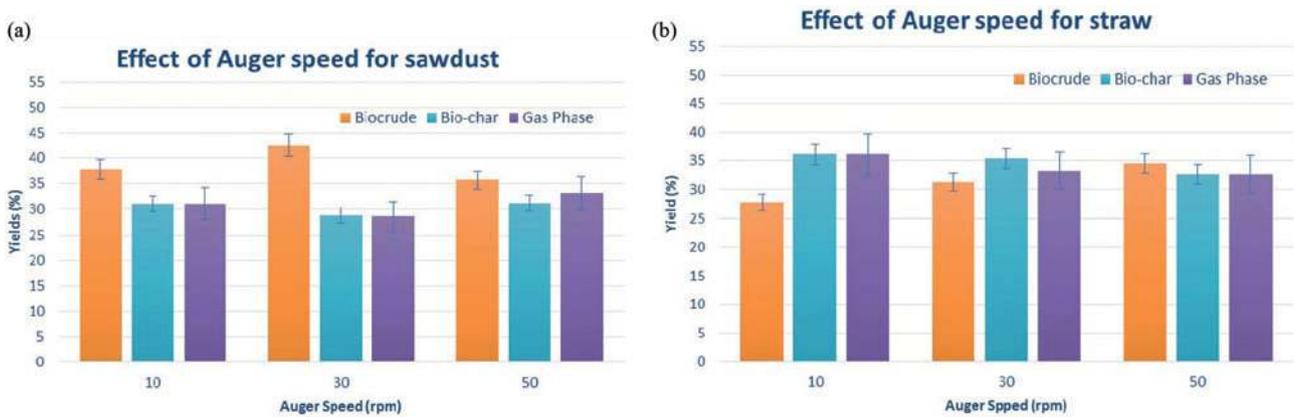
Figure 5: Effect of auger speed on yields: (a) mesquite sawdust and (b) rice straw.
