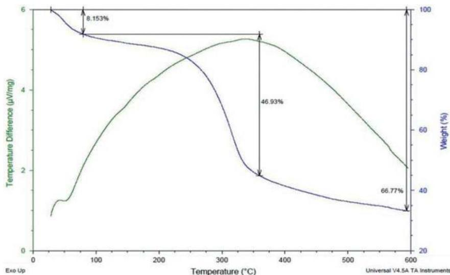
Figure 2: Thermogravimetric curves for rice straw.
