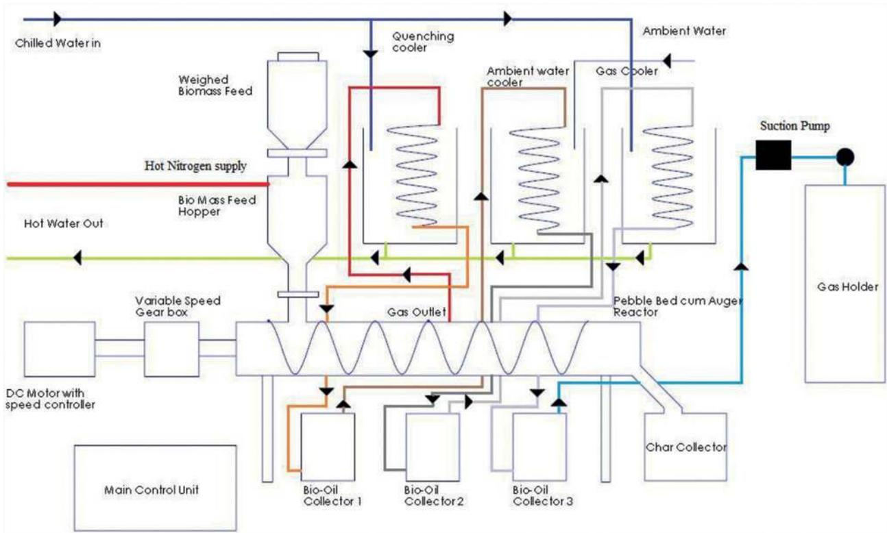
Figure 1: Schematic diagram of 500 L Auger reactor.
