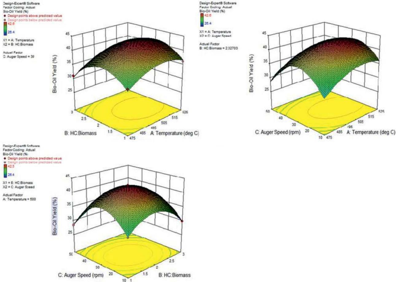
Figure 6: 3D contour plots from bio-crude production from mesquite sawdust.
