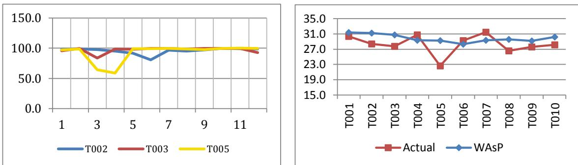
Fig. 2. (a) Machine Availability monthly variation for T002, T003 and T005, (b) WAsP-predicted and actual generation at centum MA and GA
