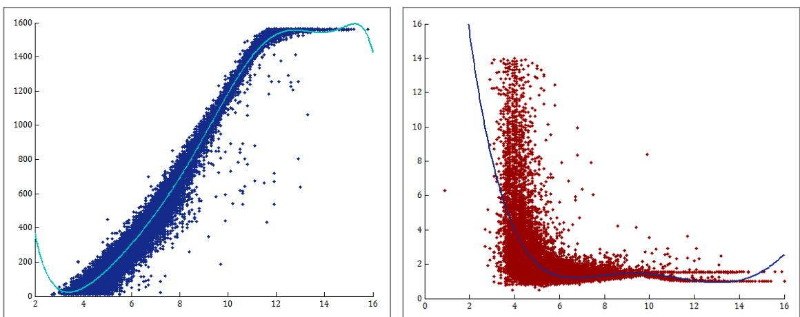
Fig. 3. (a) Actual Power Generation for T002 versus Wind Speed showing fitted polynomial, (b) Plot of  $\eta$  versus Wind Speed for T002
