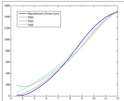
Fig. 4. Power Curves for RPCM (Power Generation in kW, Wind Speed in ms<sup>-1</sup>)
