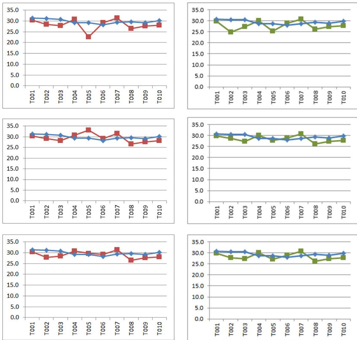
Fig. 5. Left: Actual (red) versus WAsP (blue) annual generation for centum MA and GA obtained using coarse extrapolation (top), EFM (middle) and MCM (bottom) | Right: Actual (green) versus WAsP (blue) annual generation for centum GA obtained using coarse extrapolation (top), TSPC (middle) and Reference Power Curve (PC) method.
