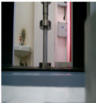
**Figure 3.** Quasi static compression test setup, sample held between two flat rigid compression plates.
