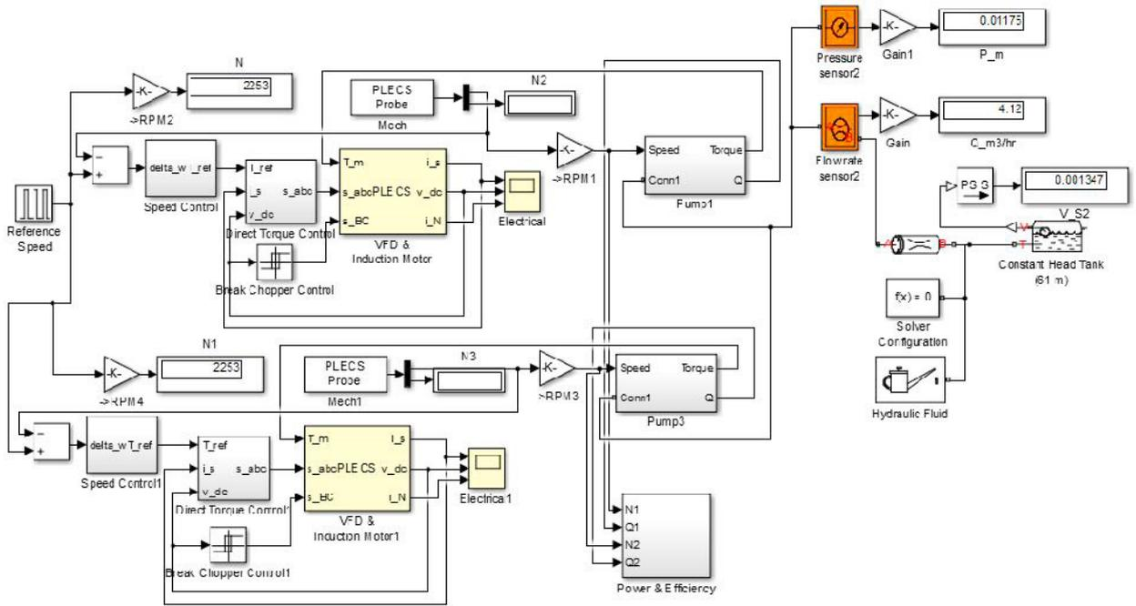
Fig. 3. PLECS modelling- Parallel pumping system
