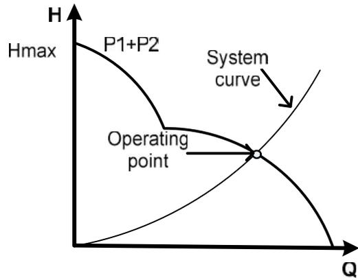
(d) Resultant performance curve with system curve (Dissimilar pumps)
