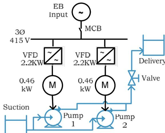
**Fig. 2.** Multi pump system connected in parallel
