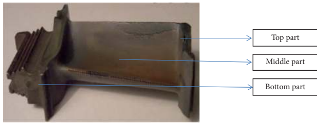
FIGURE 42: The 3-part division of the turbine blade.
