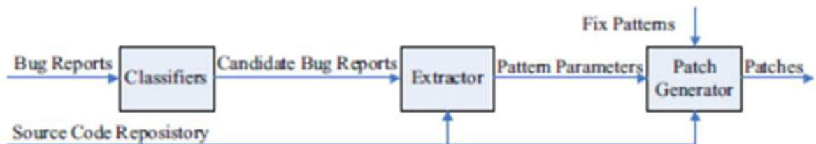
Fig 7. The Architecture of R2Fix
